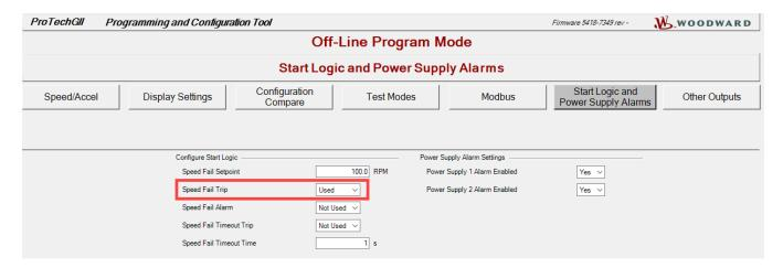
It is recommended that on ProTech TPS or MSM products, the option Speed Fail Trip always be set to "Used" whenever the configuration of the speed input probe type is "Active". If this is not desired, due to a need to have other Safety Instrumented Functions (SIF) protected in all 3 kernels, then use the "Speed Redundancy Management" option and configure both "Base Function" and "Fallback Function" to be HSS.
