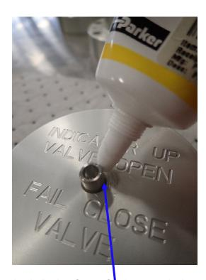
Apply Parker Super O-lube or equivalent silicone-based lubricant to the exposed surface of the VPI rod and to where the rod enters the cover. Spread the lubricant across the rod surface with a finger leaving a thin film. Wipe off excess lubricant from the cover surface.
