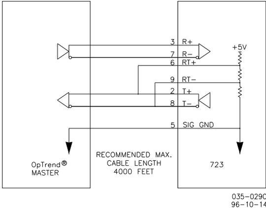
Figure 2-7. 723 RS-422 Connections with Optional Termination at Transmitter
