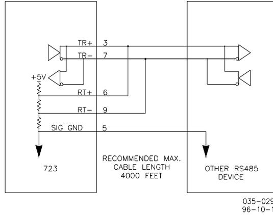
Figure 2-8. 723 RS-485 Connections with Optional Termination
