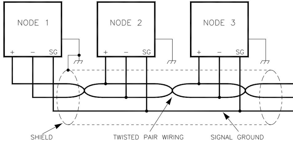
Figure 2-9. Preferred Multipoint Wiring Using Shielded Twisted-pair Cable with a Separate Signal Ground Wire
