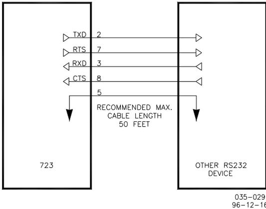
Figure 2-5. 723 RS-232 Connections
