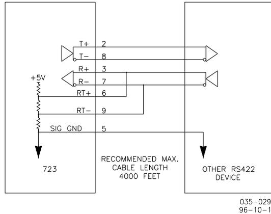
Figure 2-6. 723 RS-422 Connections with Optional Termination at Receiver
