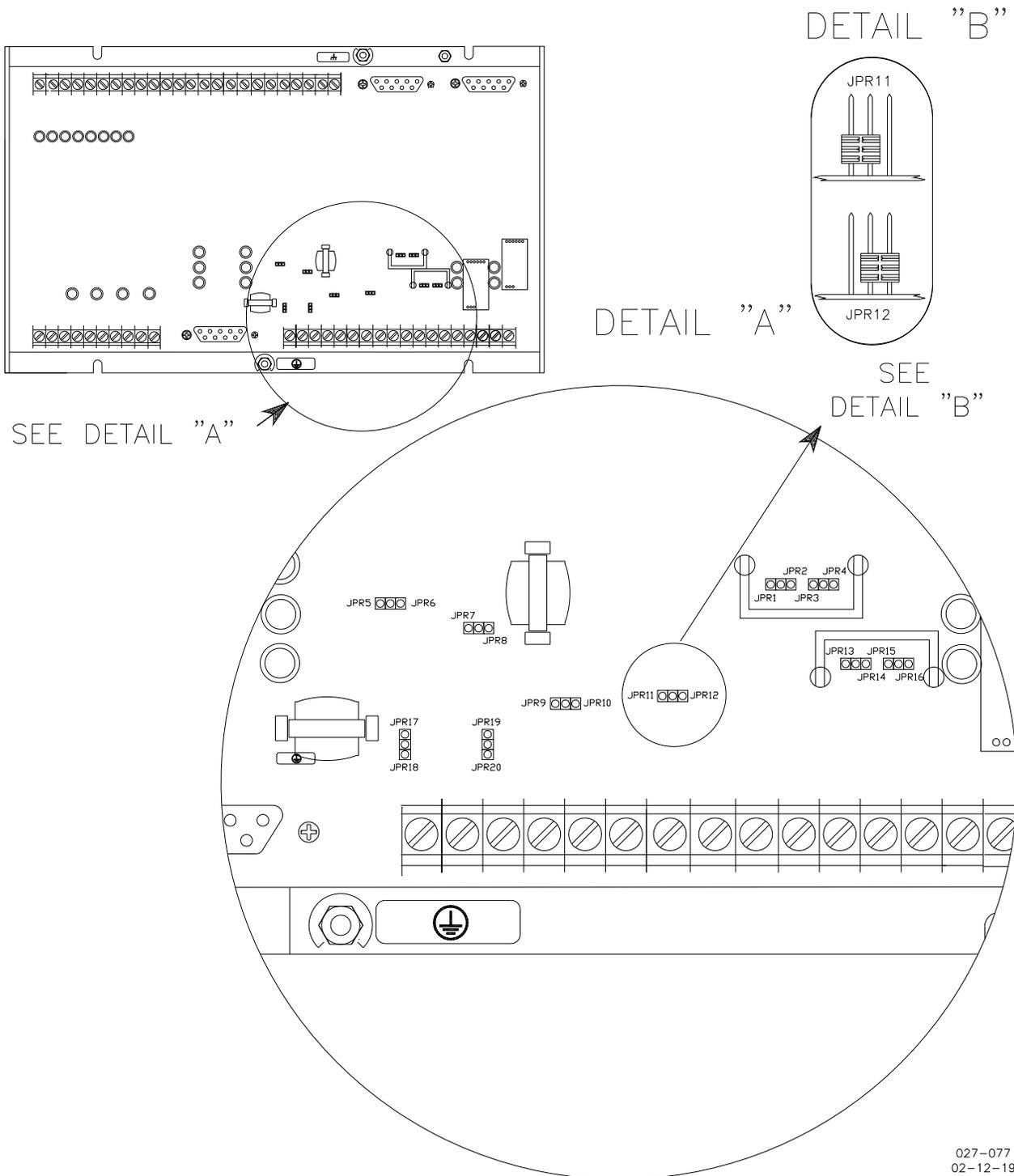
Figure 2-1. 723 Control Internal Jumpers
