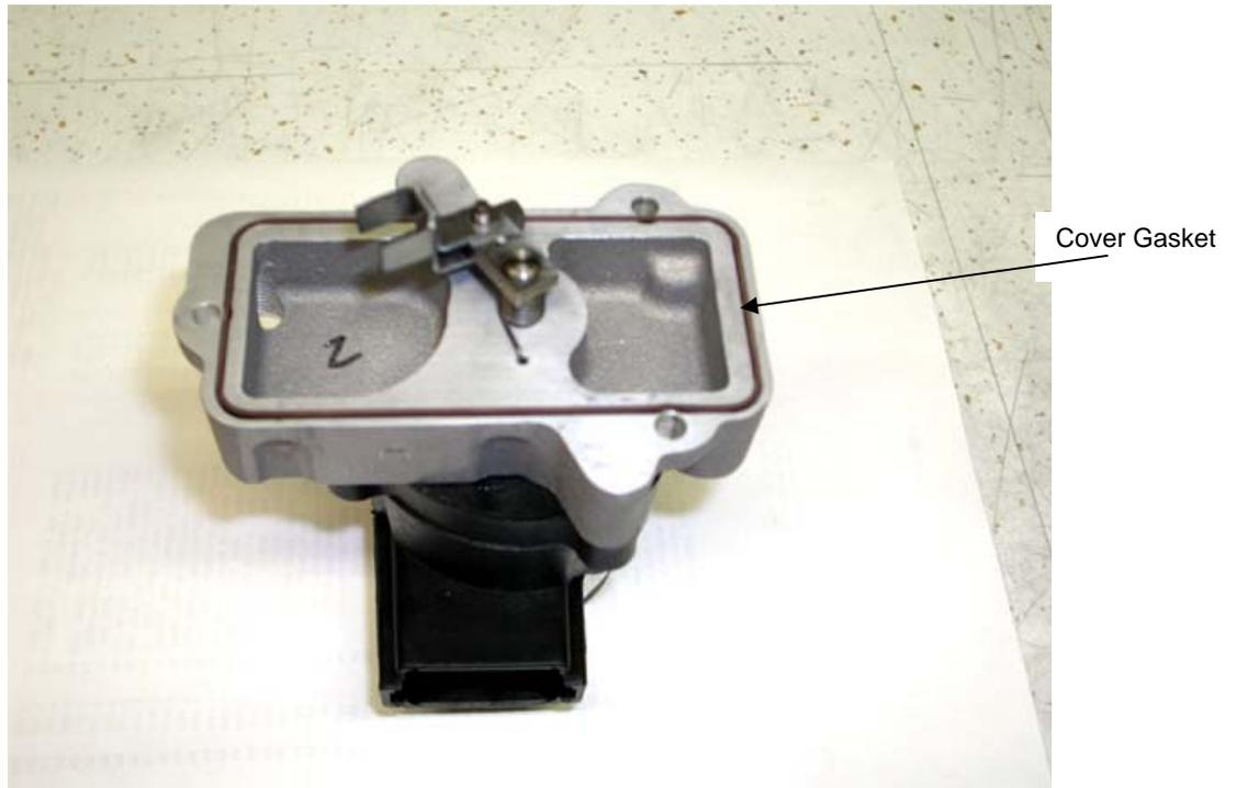
Install the new cover, with the linkage oriented as shown in the following photo. Do not force the cover into place—if the linkage is properly aligned, it will fit without being forced. The second photo, with the side walls removed, show proper cover assembly fork engagement to the pump linkage with the cover in place.
