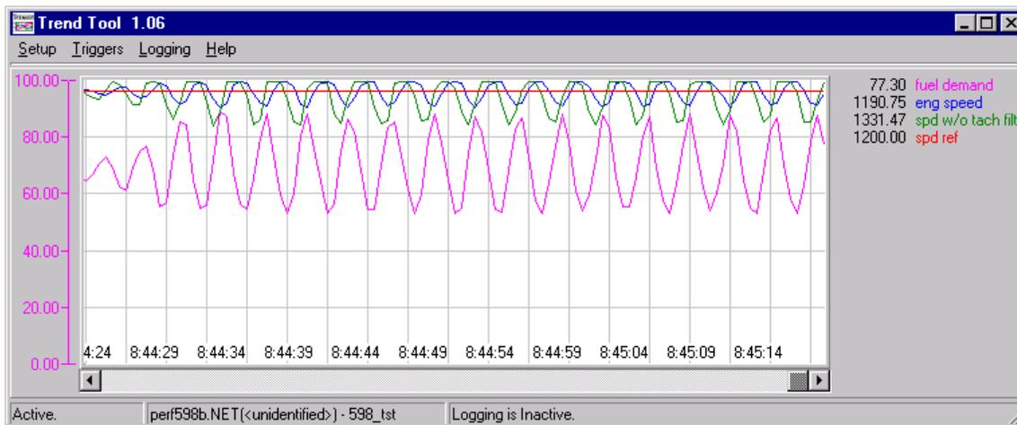
11. After recording the speed oscillations for 30–60 seconds, reduce the gain to stop the oscillations.
