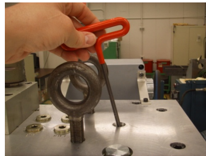
Figure 3-3. Adjusting Needle Valve
