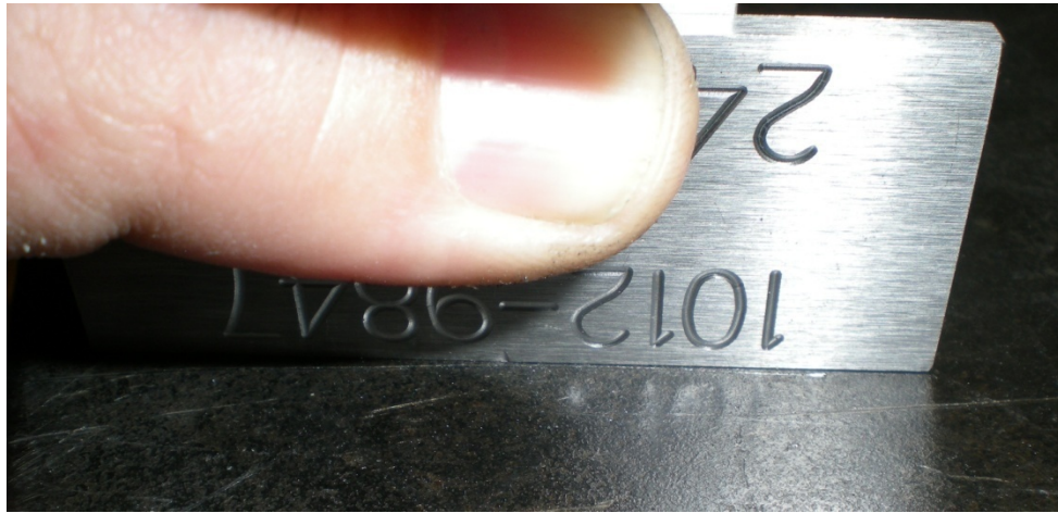
Figure 3-17. Aligning Scribe Mark in Yoke with Rigging Tool & Extender Block
