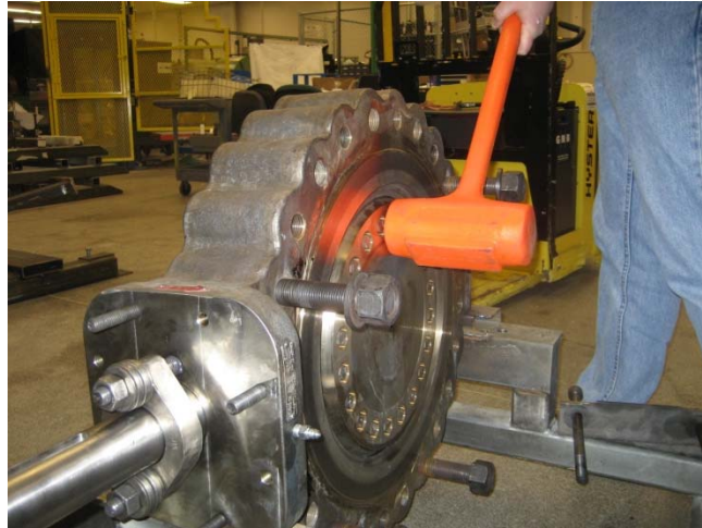
Figure 3-13. Adjusting Valve Seat Gap
