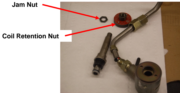
Figure 3-6. Disassembled Trip Solenoid Assembly
