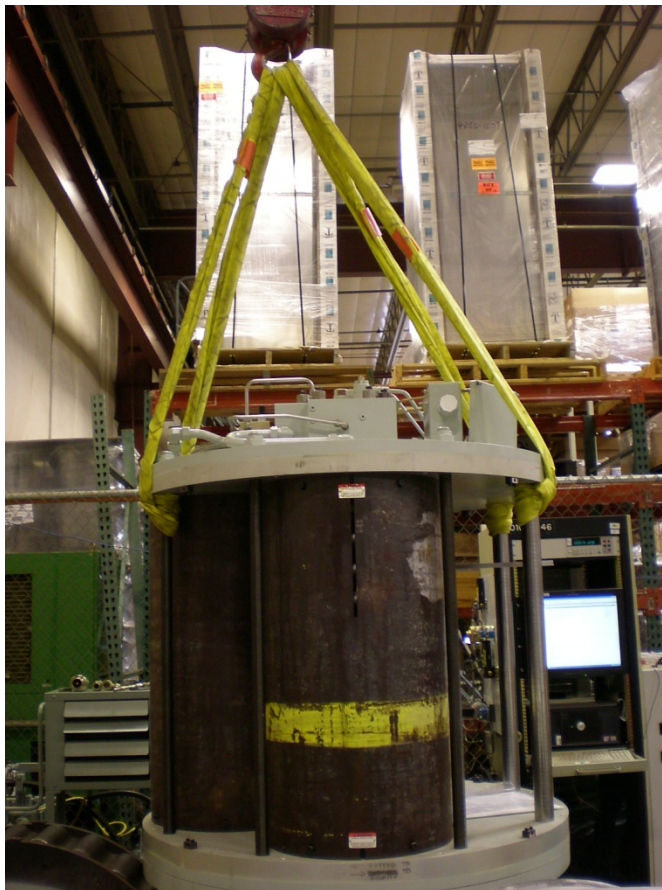
Figure 3-9. Actuator Rigged via Tie Rods for Lifting
