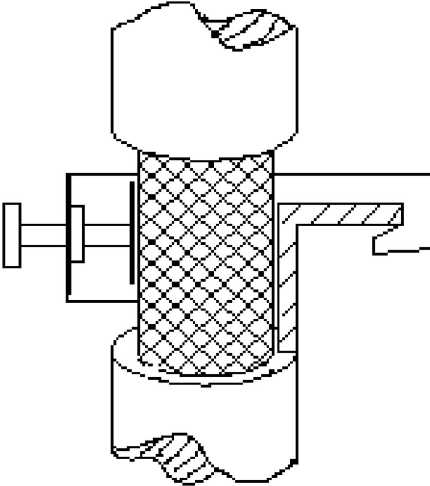
Figure 5-3. Strain Relief and Grounding
