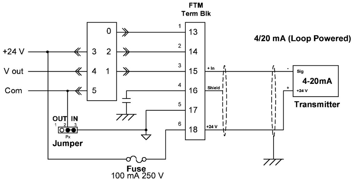
Figure 5-7. Example Wiring Diagram - Loop Powered 4–20 mA Signal to Dataforth FTM
