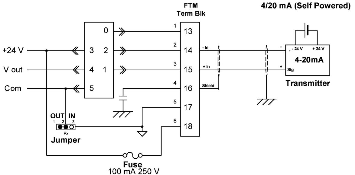
Figure 5-8. Example Wiring Diagram - Self-powered 4–20 mA Signal to Dataforth FTM
