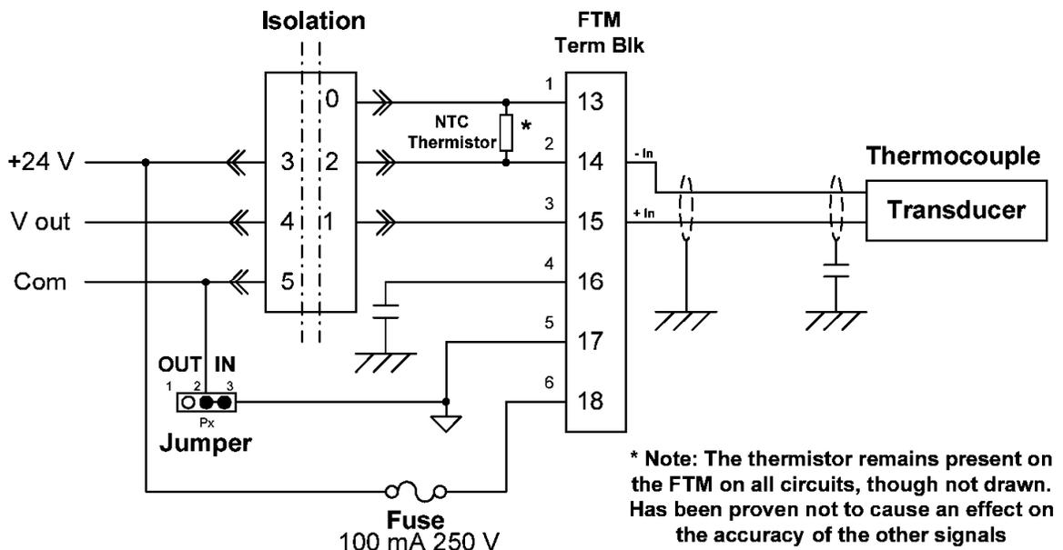
Figure 5-5. Example Wiring Diagram—Thermocouple to Dataforth FTM
