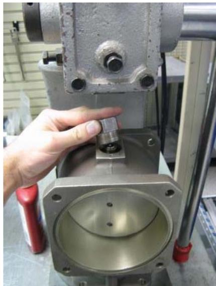
9. Install spring seats, loading spring, lower bearing, and retaining ring
