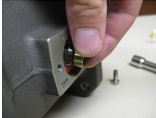
7. Hold shaft firmly compressing the spring, remove remaining plate bolt and slowly remove shaft from unit.
