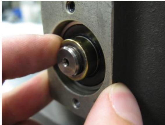
7. Install outboard retaining ring to secure bearing in place and allow loading of the shaft [8535-300 1x 5H-9899 (1017-513), 346-8987 1x 354-2662 (1017-355)].
