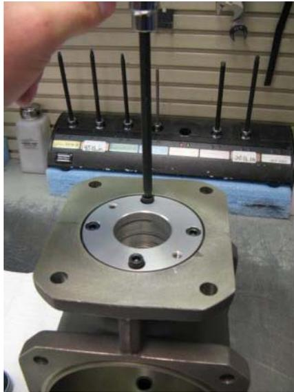
2. (346-8987 Only) Install outboard seal into valve housing [1x 149-2091 (1355-109), 1x 354-2661 (1382-1086), Assembled in Step 3.4.1]
