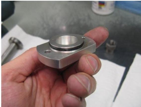
13. Install top cap with O-ring onto valve assembly.
