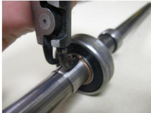
9. Remove bearing from shaft [1x 5P-6836 (180061)].
