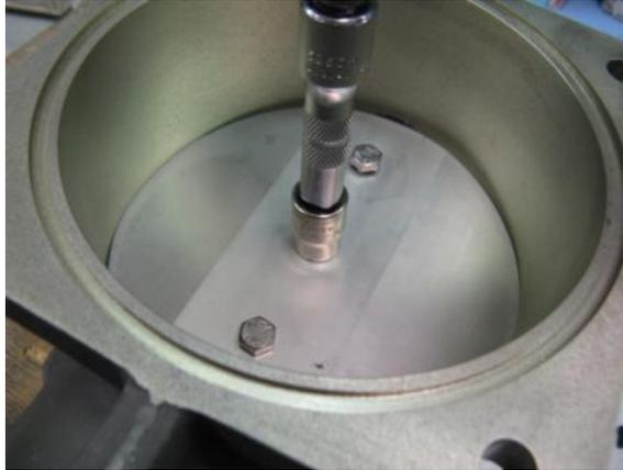
11. Again (Same as step 8) Press outboard bearing to ensure bearing did not shift during prior operations [Tool: 1008-4106 Simplified (Steel Tube: O.D. 1.050-1.100, I.D. 0.900 min), arbor press].
