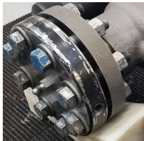
Figure 3-2. Illustration of Raised Face Style Diverging Sleeve
