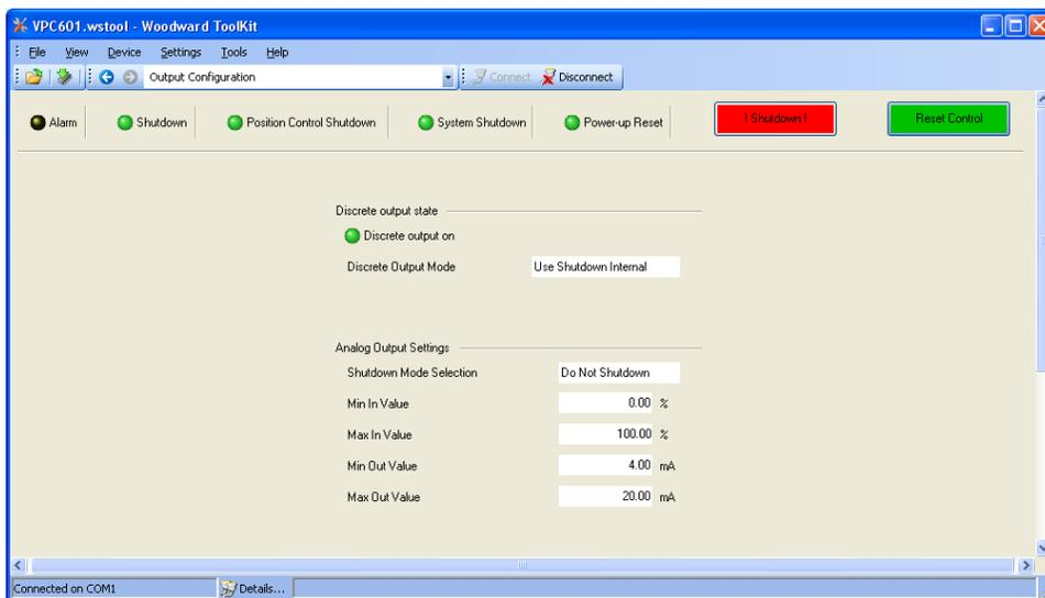
Figure 4-22. Output Configuration
