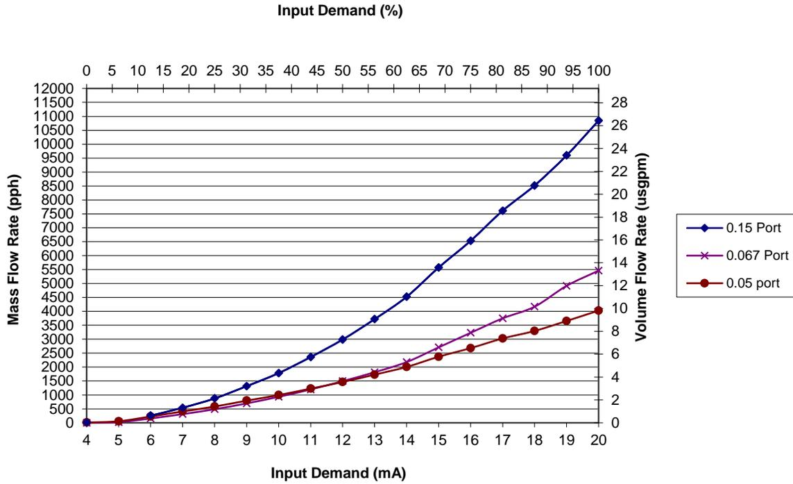
Figure 6-1. Metering Port Size—0.82 Specific Gravity
