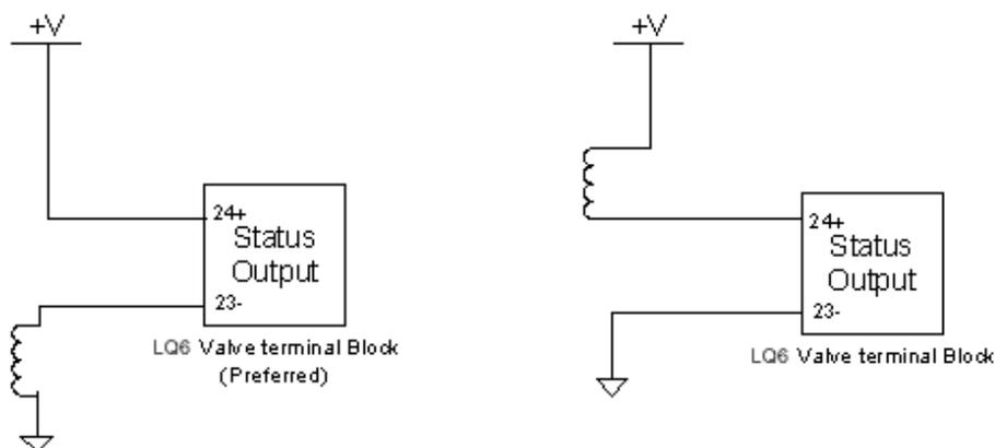
The two methods for wiring the Status Output are shown above. The Status Output indicates if the LQ6 is shut down or running. There are two ways for the LQ6 to be shut down—if the Shutdown/Reset input is in shutdown, or if a diagnostic has been triggered. If the LQ6 is in a shutdown situation, the status output is open (no current).
