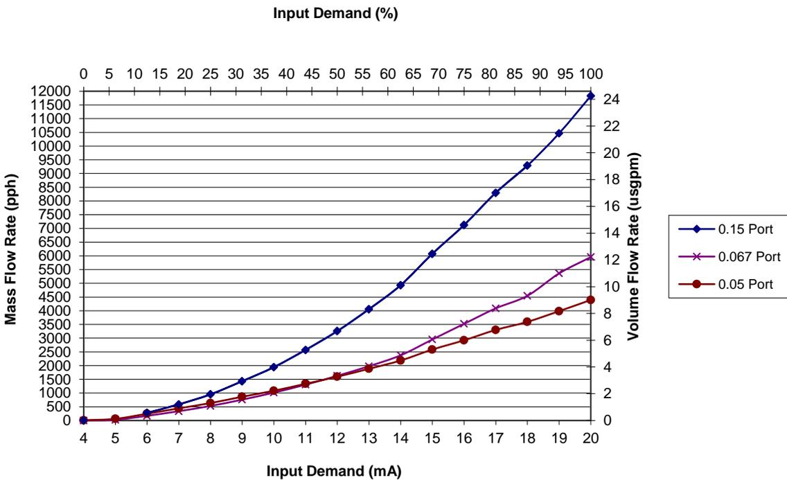
Figure 6-2. Metering Port Size – 0.975 Specific Gravity
