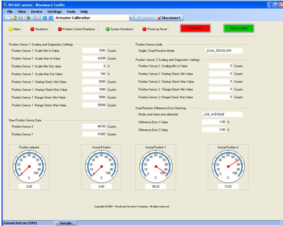
Figure 4-21. Dual Resolver Actuator
