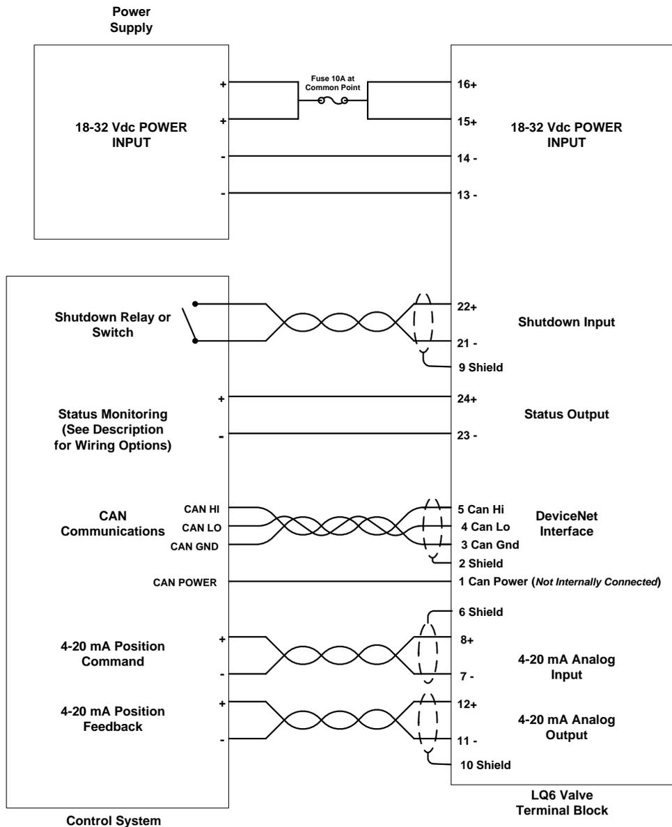
Figure 2-3. LQ6 Plant Wiring Diagram
