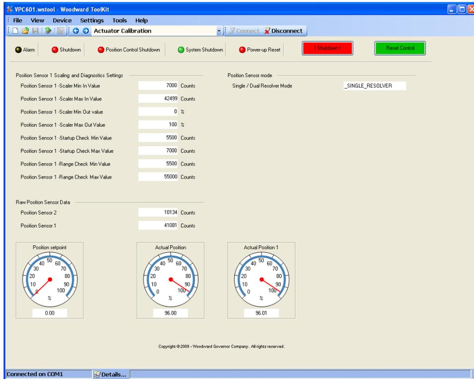
Figure 4-20. Single Resolver Screen
