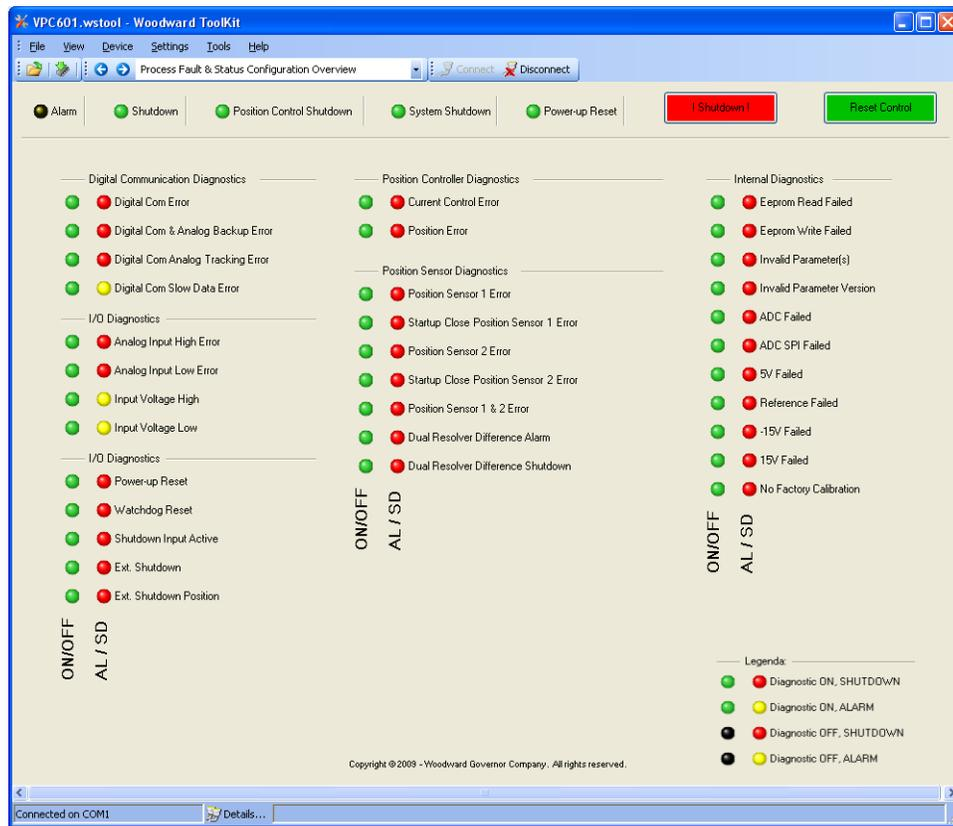
Figure 4-14. Process Fault &amp; Status Configuration Overview
