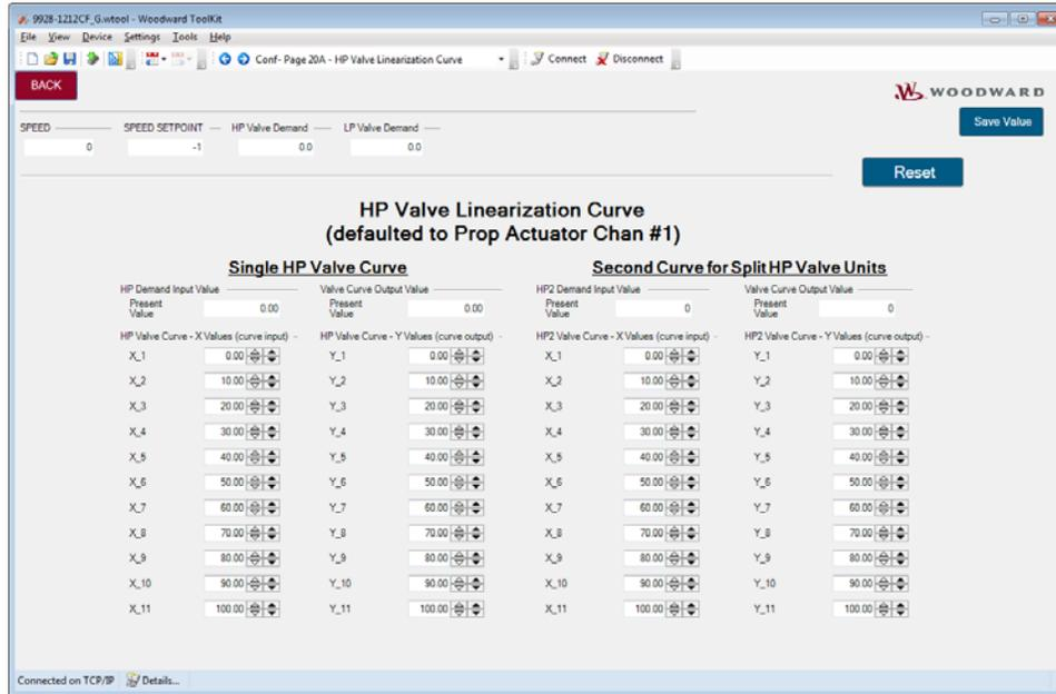
Figure 3-44. Service HP Valve Linearization Curve
