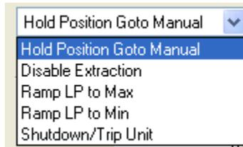
When an extraction/admission/E/A sensor is detected faulty, then the control will decide the strategy to apply based on this settings:
