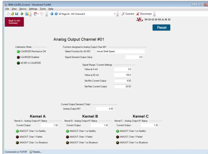
Figure 4-12. Service Analog Output Details
