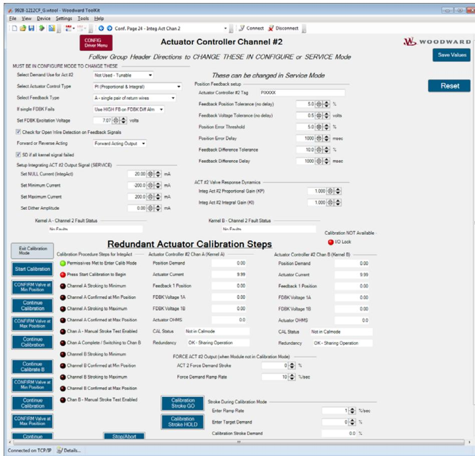
Figure 3-43. Actuator Controller Driver Channel 2
