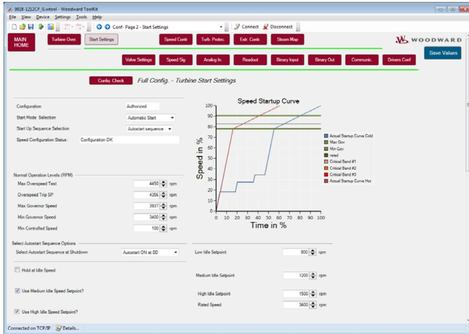
Figure 3-6. Turbine Automatic Start Settings
