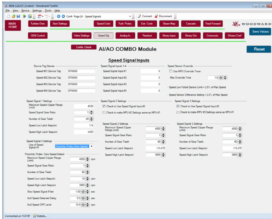
Figure 3-27. Speed Signal Settings
