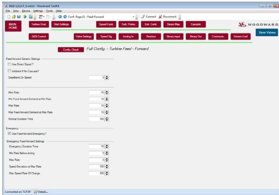
Figure 3-24. Feed-forward Performance Control
