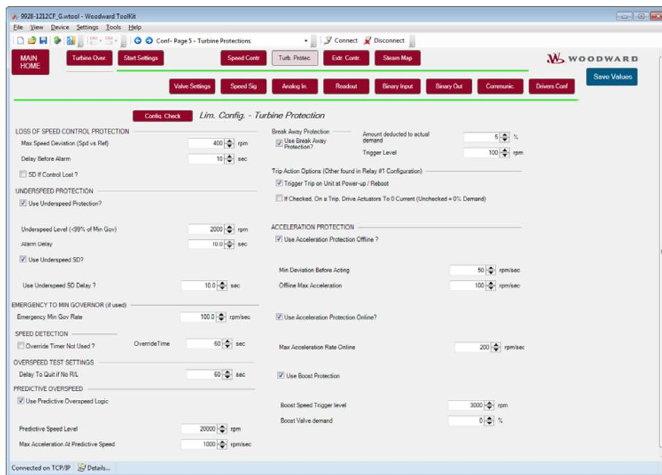
Figure 3-12. Turbine Protection
