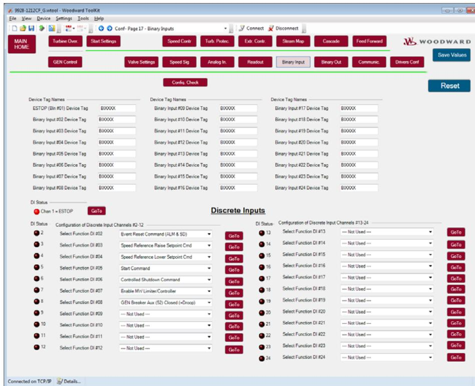
Figure 3-32. Discrete Input Settings
