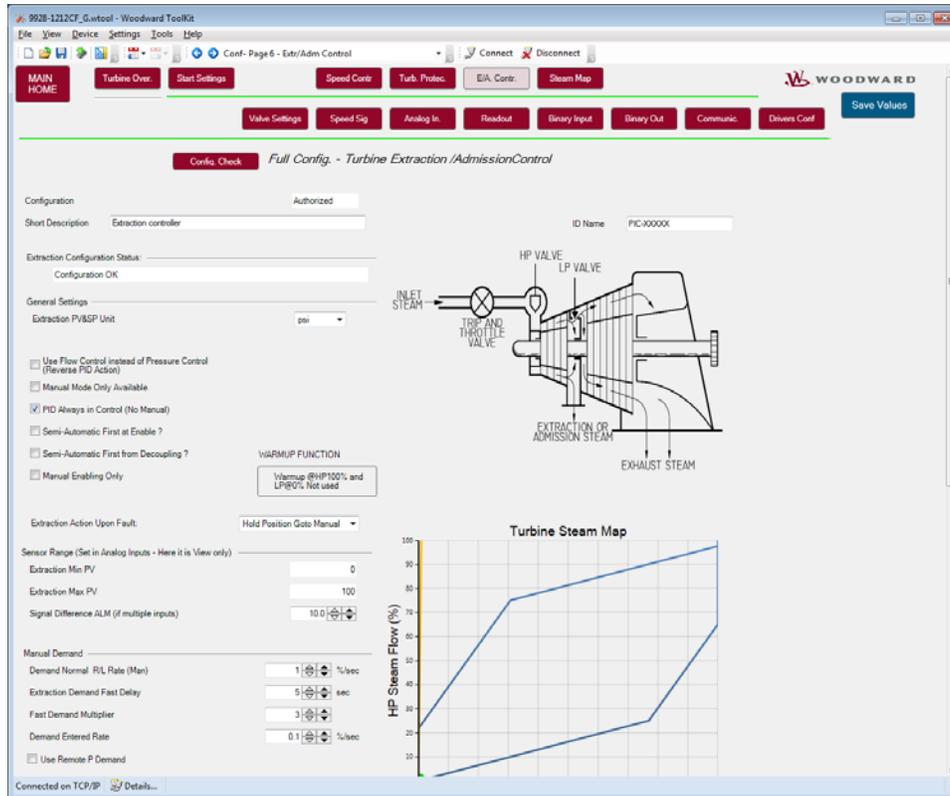
Figure 3-14. Turbine Extraction/Admission Control (bottom half)
