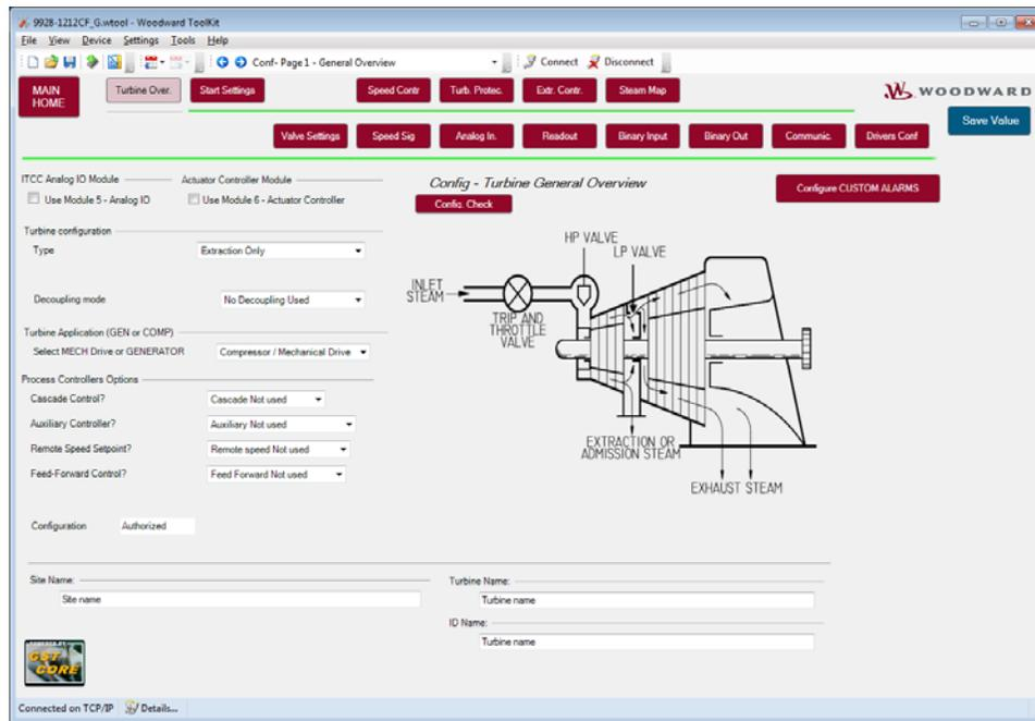
Figure 3-3. Turbine Overview Minimal Example (Single Valve)
