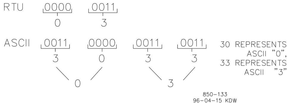
Figure 8-1. ASCII/RTU Representation of 3
