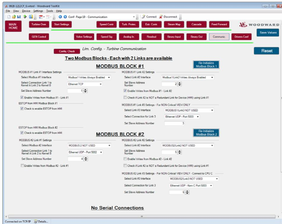
Figure 3-37. Communication (MODBUS) Settings
