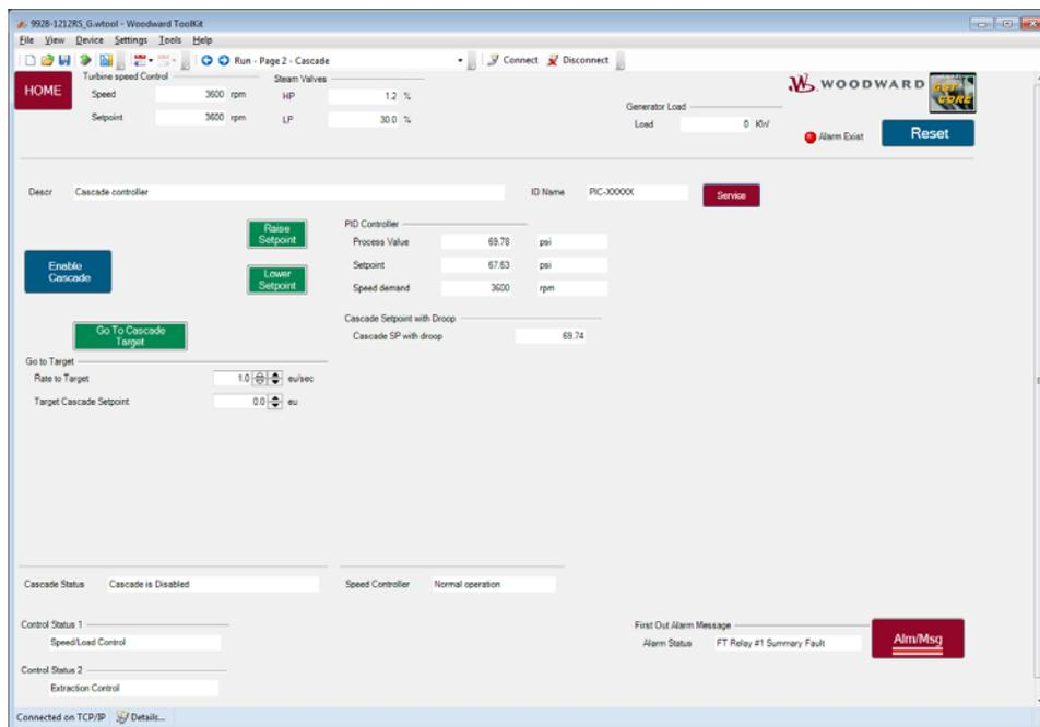
Figure 5-13. RUN Cascade Control
