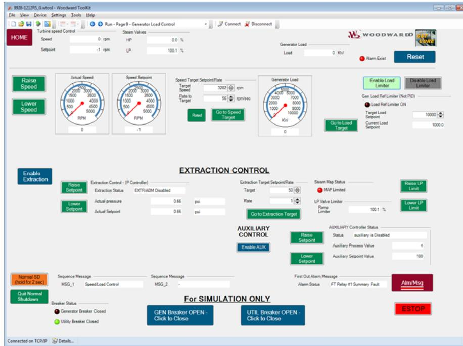
Figure 5-16. Extraction Turbine w/ AUX limiter (Generator)
