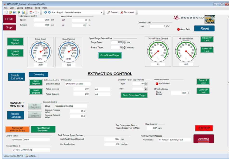
Figure 5-7. Start/Run at Rated Speed (Extraction and Cascade configured)
