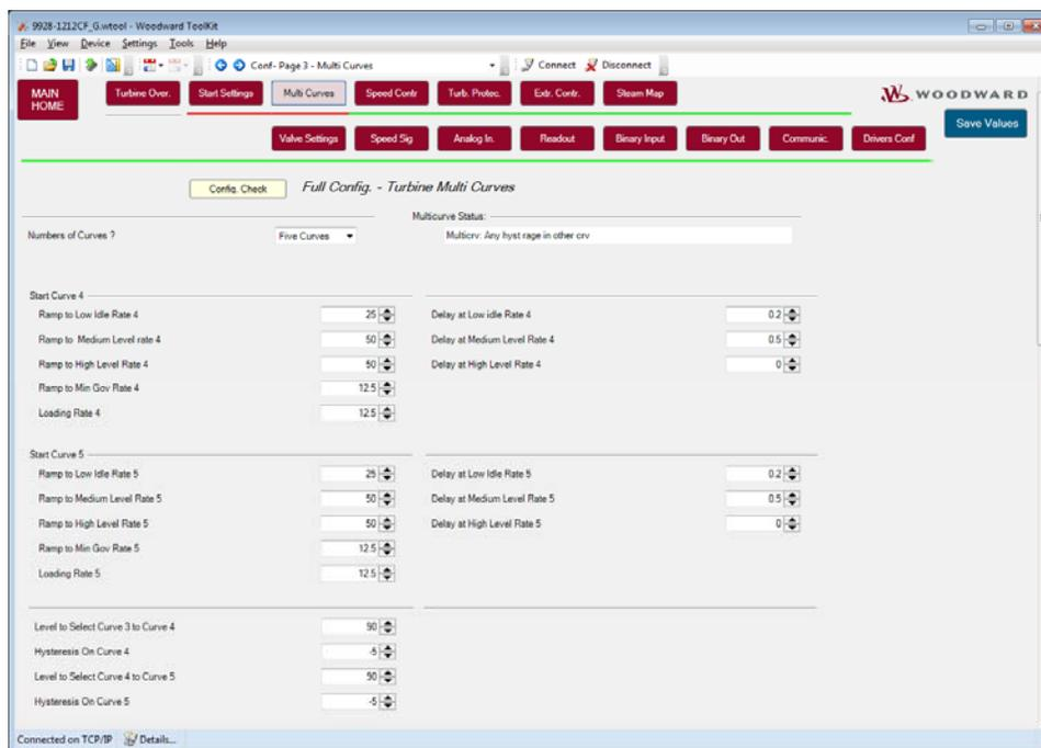
Figure 3-10. Multi-Curve Hot/Cold Settings (5 curve example)
