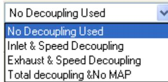
This application option is only visible when configured for extraction, admission, or extraction/admission turbine types. The ratio/limiter logic controls the interaction of both HP and LP valves to control the desired turbine related parameters (i.e. speed, extraction pressure/flow, inlet pressure/flow, exhaust pressure/flow) and minimize the effects of one controlled process on the other controlled process.
