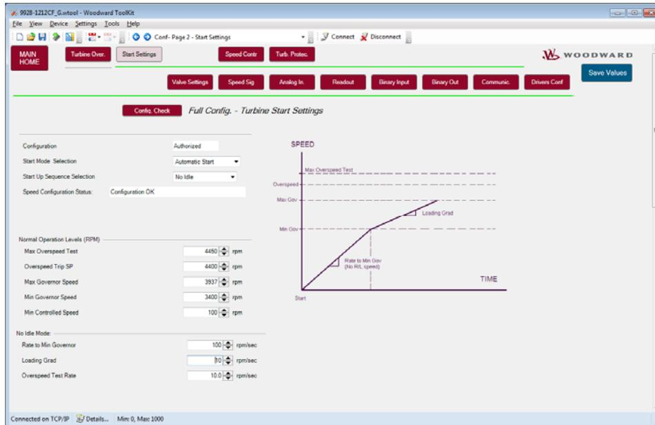
Figure 3-8. Turbine No Idle Settings
