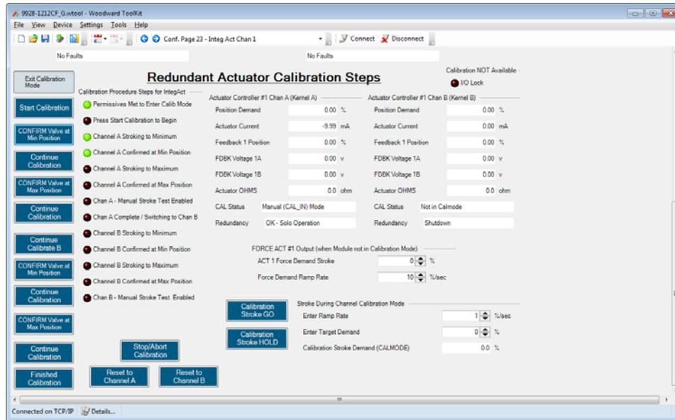
Figure 3-42. Actuator Controller Driver Channel 1 - Calibration
