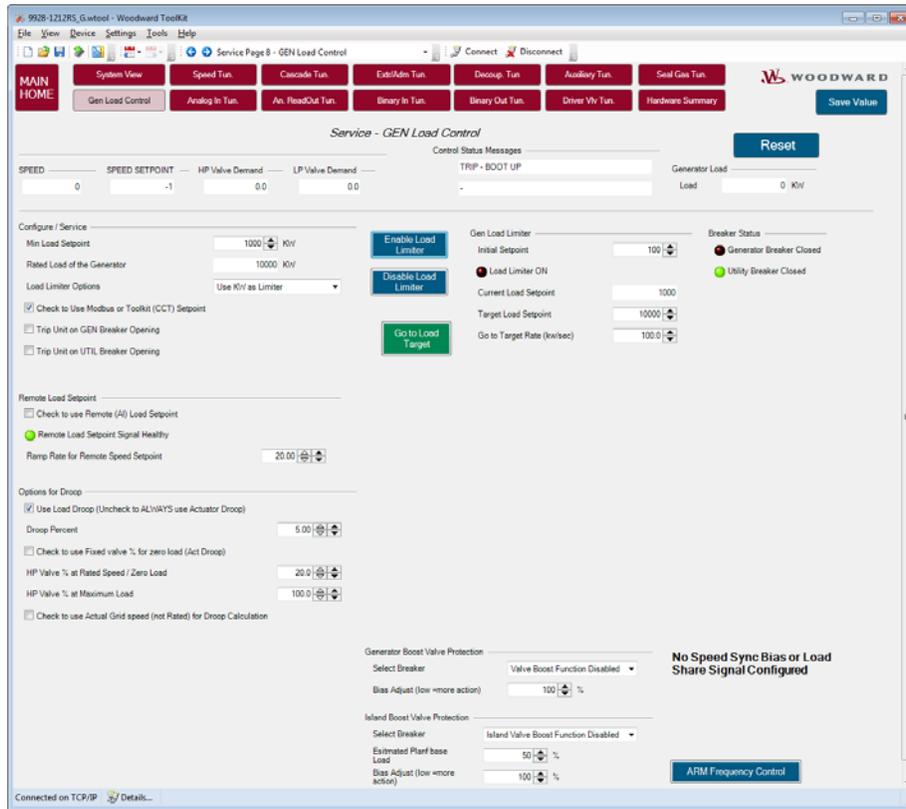
Figure 4-8. Generator Load Control Tuning
