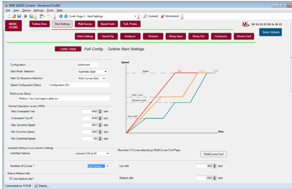
Figure 3-9. Turbine Multi Curve Settings
