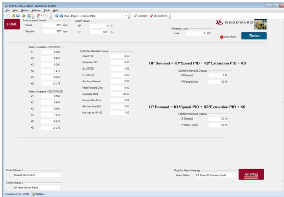
Figure 5-11. PID/Valve Demand Calculations
