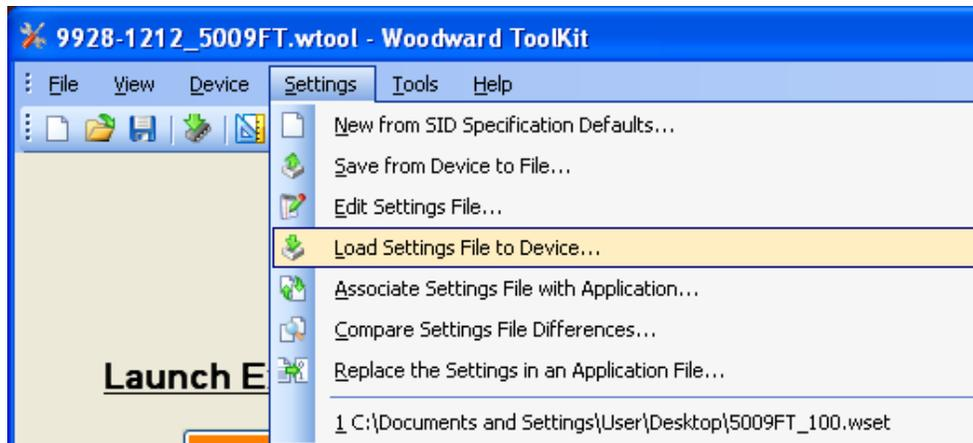
Figure 6-11. Load Settings into Control
