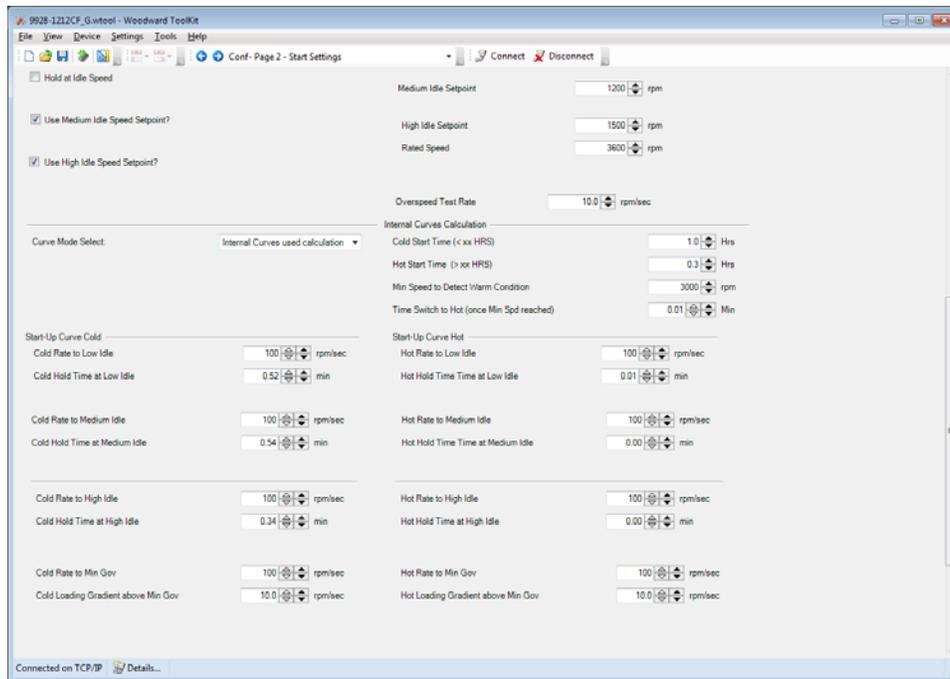
Figure 3-7. Turbine Start – Hot/Cold Settings
