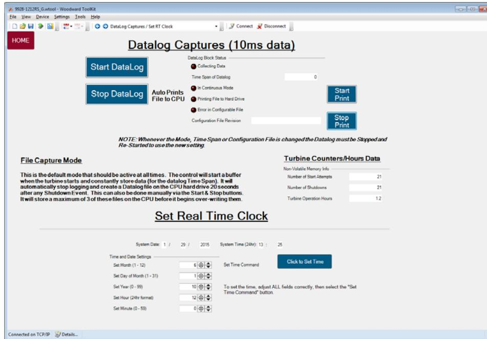
Figure 5-20. Datalog &amp; Real Time Clock Setting
