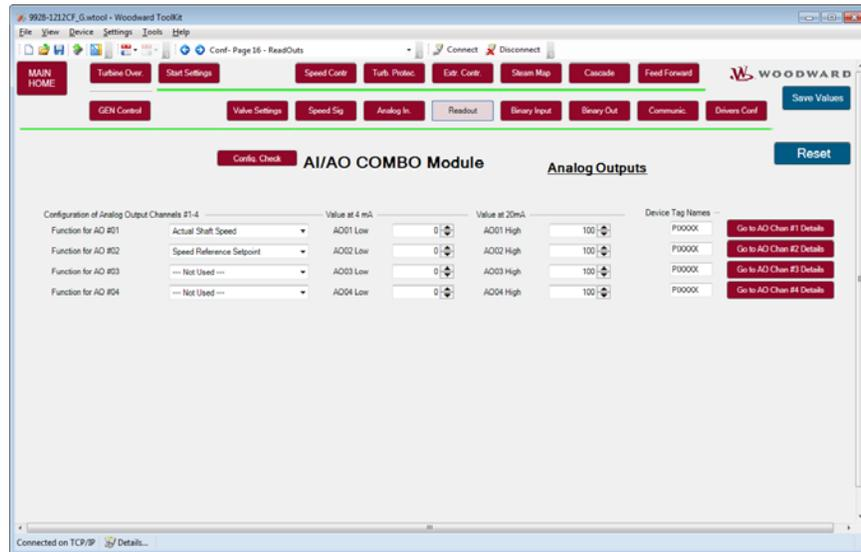
Figure 3-30. Analog Output Signal Settings
