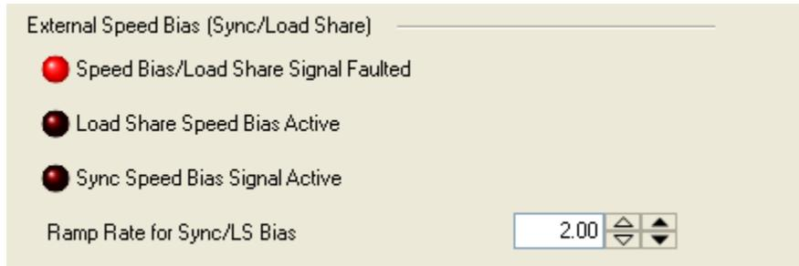
**Status LEDs** — of the Signal fault status, and whether or not the signal is actively being used for synchronization or load sharing.
