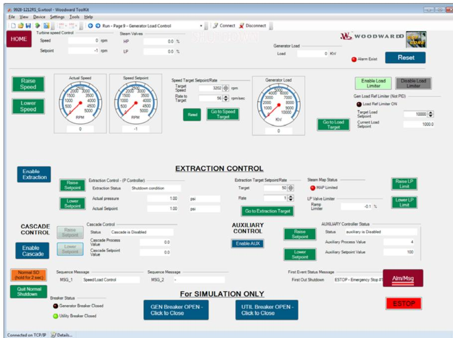
Figure 5-17. Extraction Turbine w/ CASC Controller (Generator)
