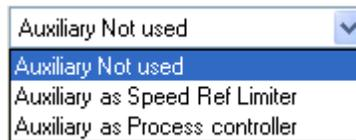
Select the Auxiliary PID's functionality by configuring it as a Limiter or a Process Controller. The Auxiliary PID can be used to limit or control generator power, plant import power (control only) \export power, turbine inlet pressure, turbine exhaust pressure, pump/compressor discharge pressure, or any other auxiliary parameters directly related to turbine speed/load.
