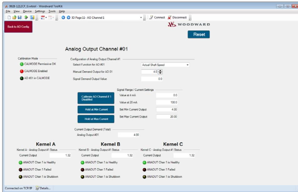
Figure 3-31. Analog Output Detailed Settings
