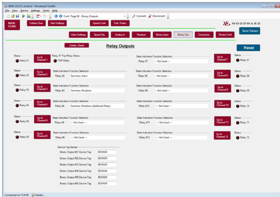
Figure 3-34. Relay Output Settings
