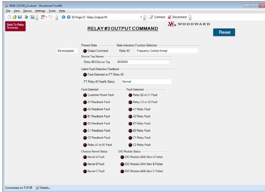
Figure 4-15. Discrete Relay Output Channel Detail
