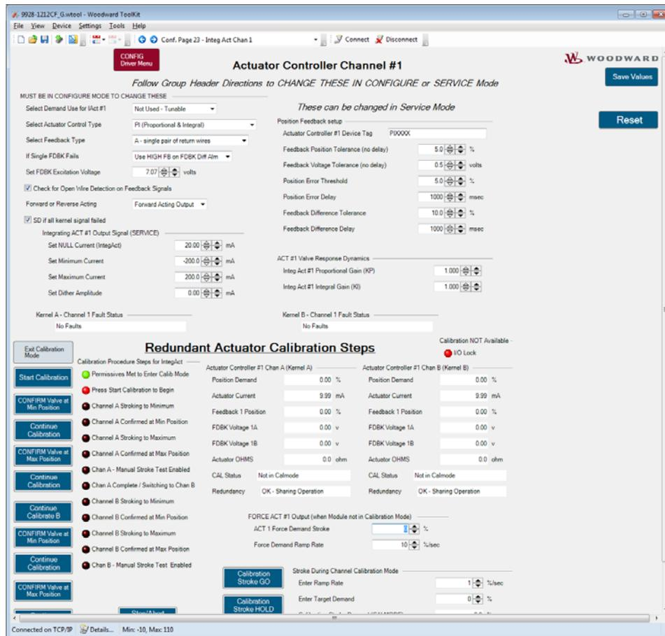
Figure 3-41. Actuator Controller Driver Channel 1
