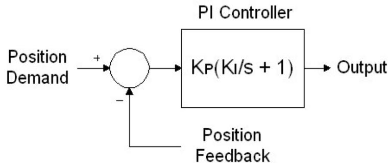
**P** – This interfacing is to an integrating actuator and its position feedback device, with only the proportional gain active in the demand vs. position control loop.
