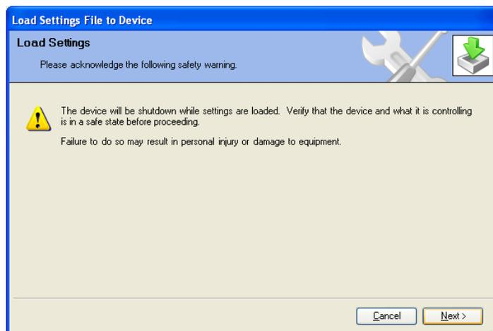
Figure 6-16. WARNING Turbine must be Shutdown
