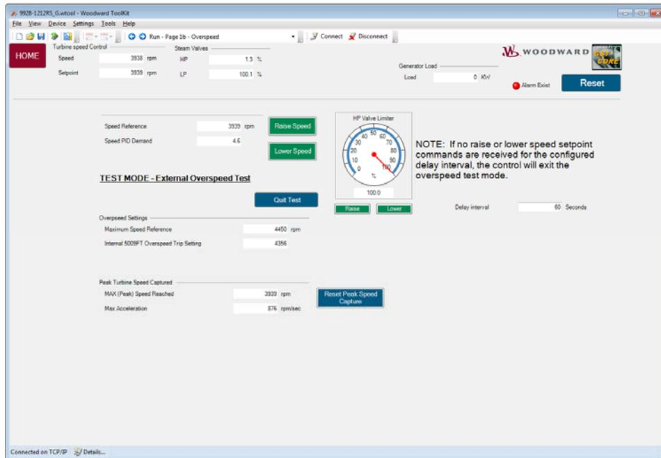
Figure 5-10. External Overspeed test
