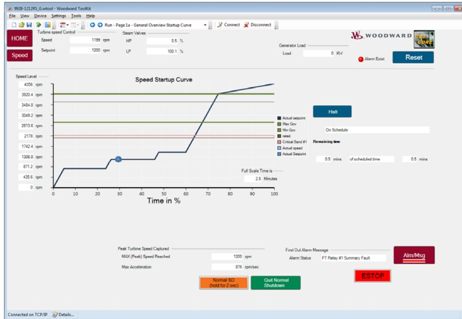
Figure 5-5. Dynamic Startup Curve
