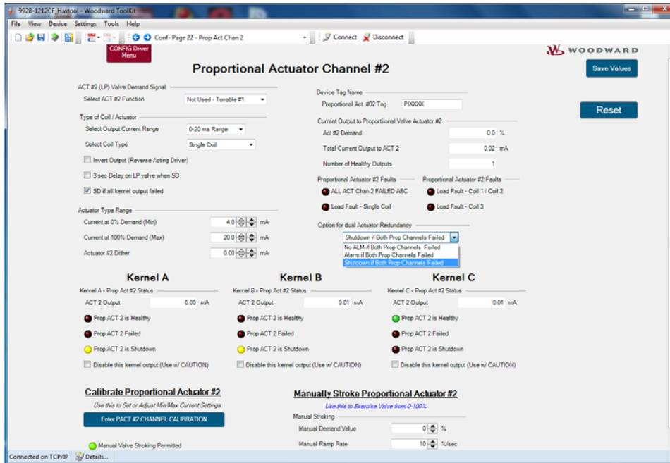
Figure 3-40. Proportional Actuator Driver Channel 2
