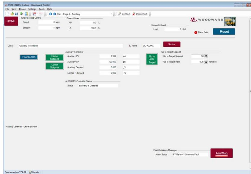
Figure 5-15. RUN Auxiliary Controller Control
