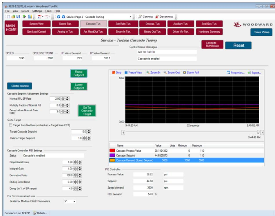
Figure 4-3. Cascade Control Tuning
