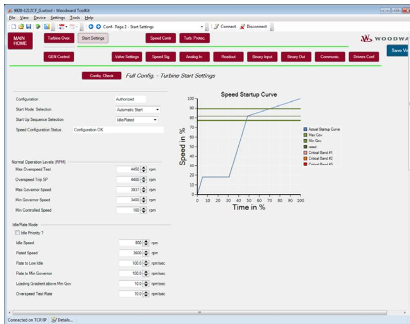
Figure 3-5. Turbine Idle/Rated Start Settings
