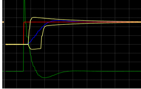
Figure 5-4. Step response test
