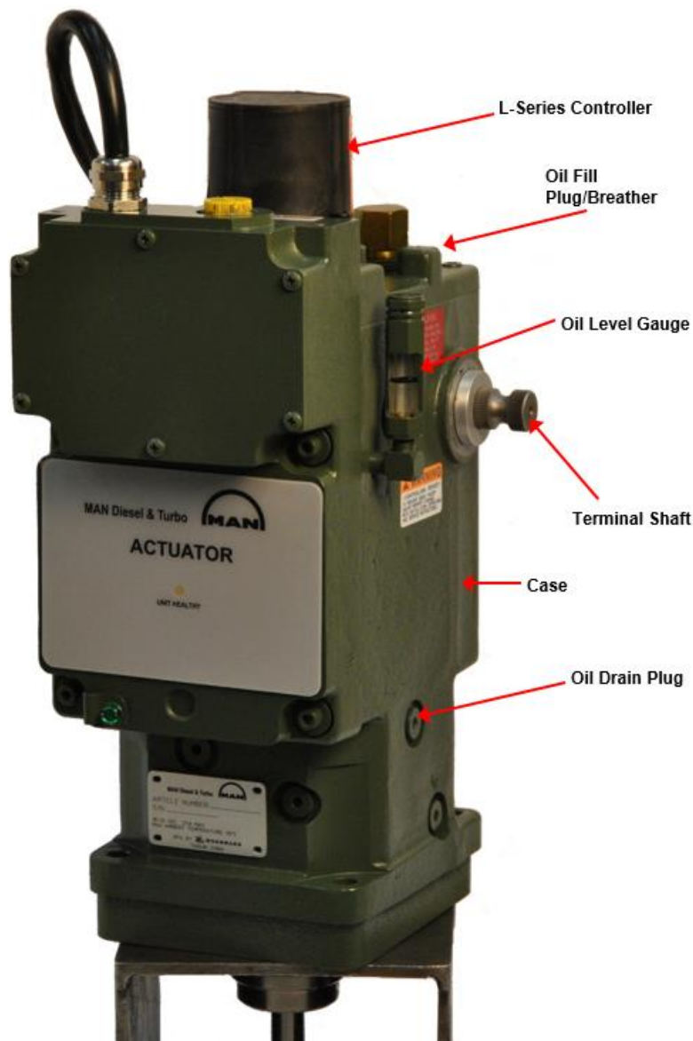
Figure 2-1. MAN Actuator Overview
