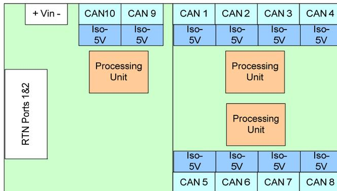
Figure 2-4. GW CAN Port Internal Configuration
