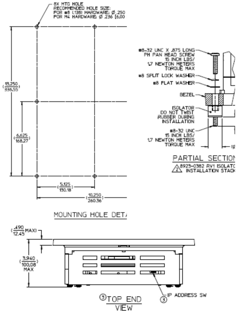
Figure 4-1. Optional RV1 Isolation Kit Installation
