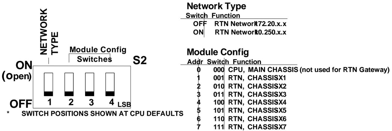
Figure 4-5. Module Configuration Switch Setting
