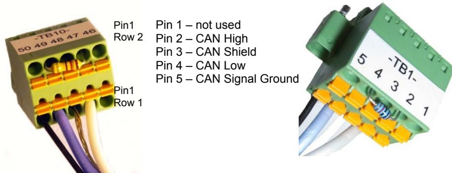
Figure 4-8. CAN Communication Ports
