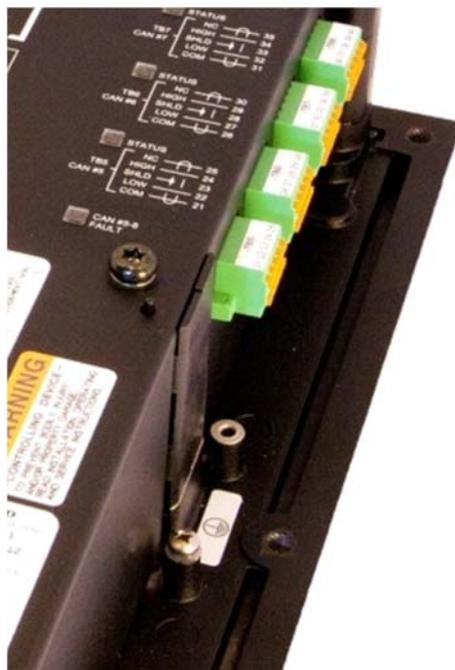
Connect Protective Earth ground (PE) to the chassis at the termination point
