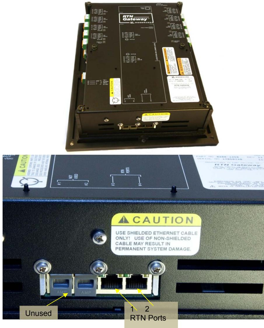
Figure 4-6. 10/100 BaseT Ethernet Ports (RJ45)
