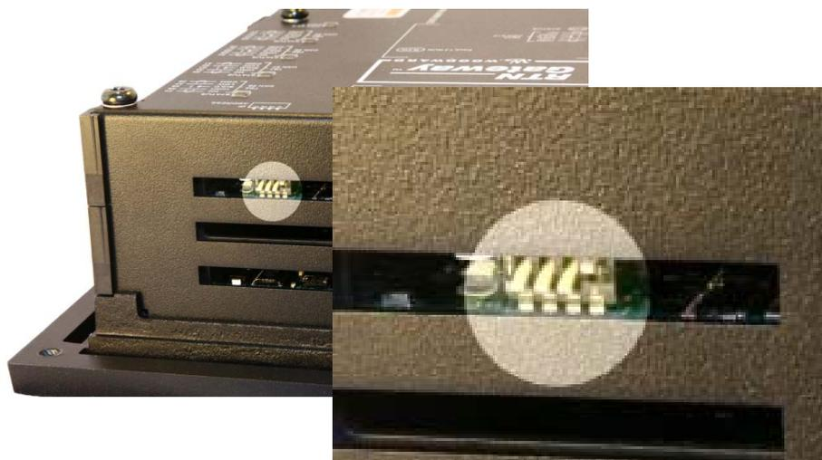
Figure 4-4. Module Configuration Switch
