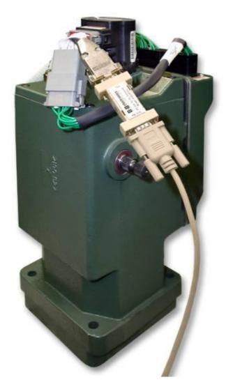
Figure 5-2a. Programming Harness Connection
