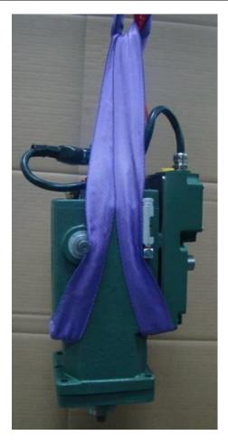
Figure 2-3. Proper Lifting Technique
