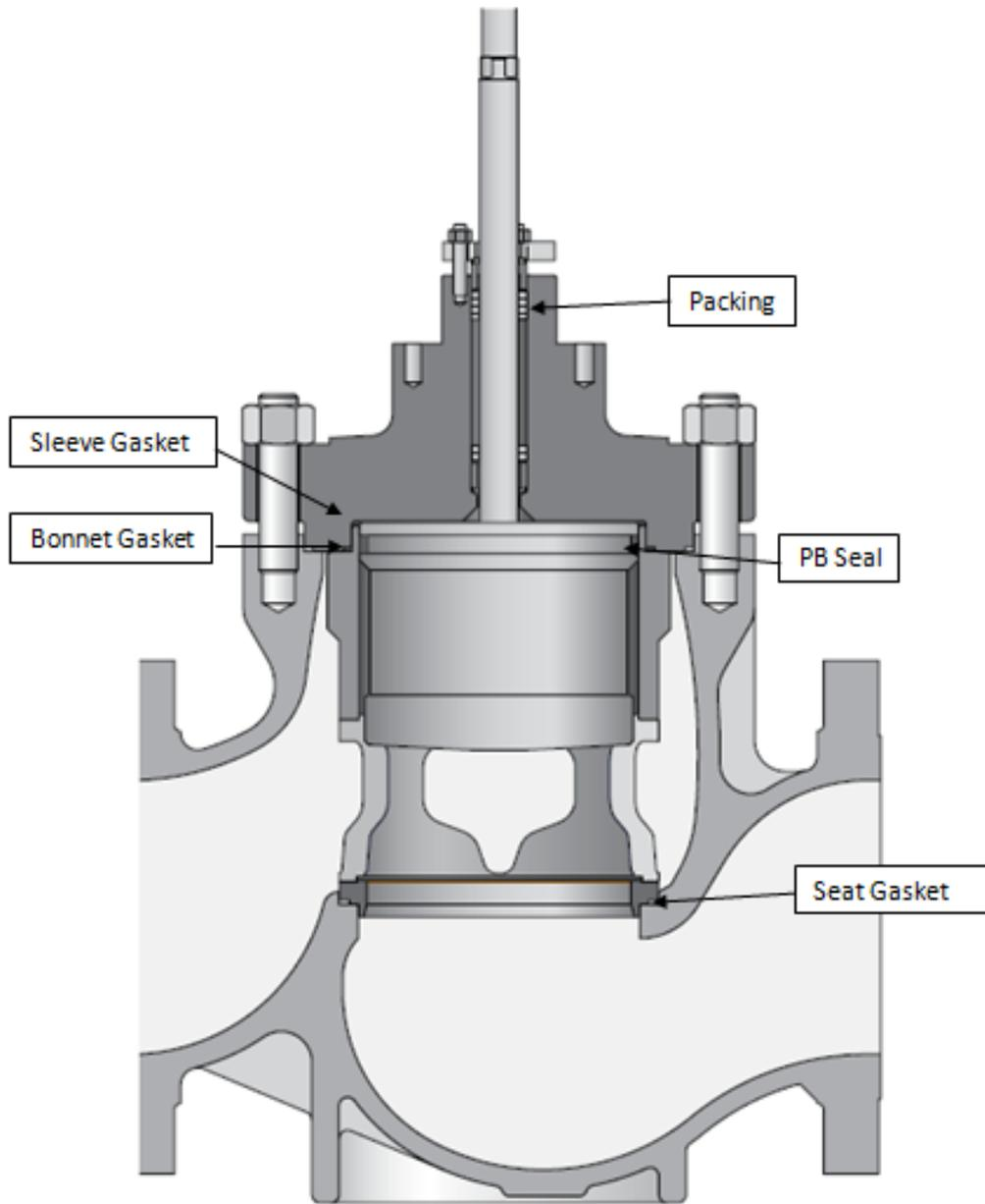
Figure 1-2. Cutaway, Metering Valve
