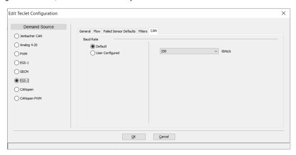
Figure 5-12a. Edit TecJet Configuration - CAN (Default)
