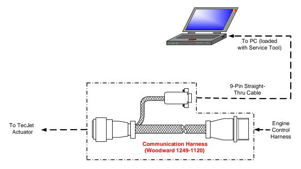
Figure 5-1. Communication- Harness Connections
