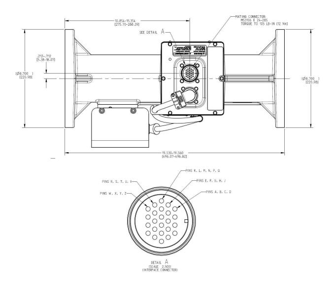
Figure 2-2a. Actuator Connector View
