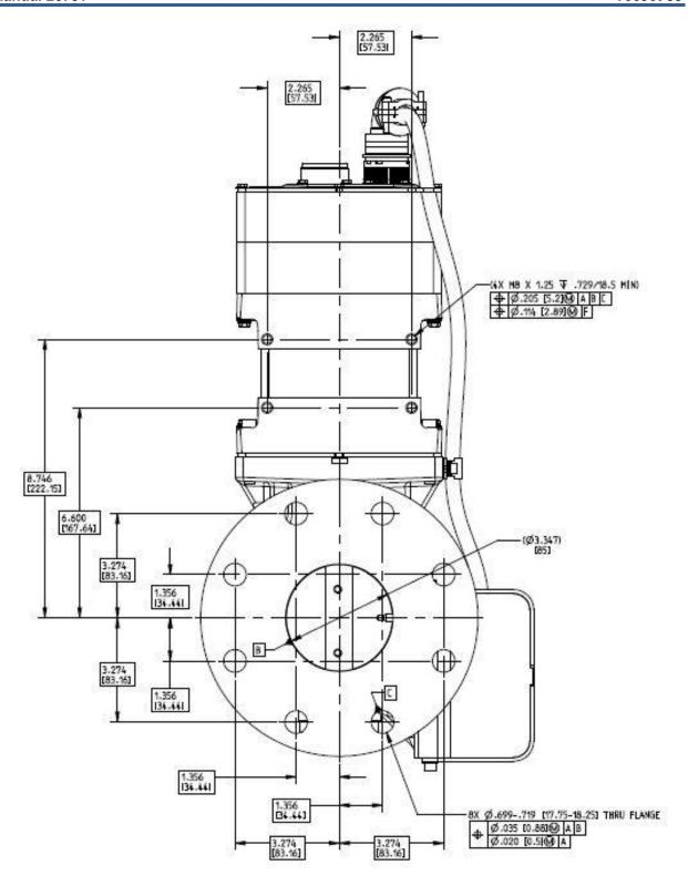
Figure 2-2b. Valve Outlet Flange and Actuator Mounting View
