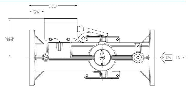
Figure 2-2e. Preferred Mounting Orientation with Actuator Positioned Horizontally
