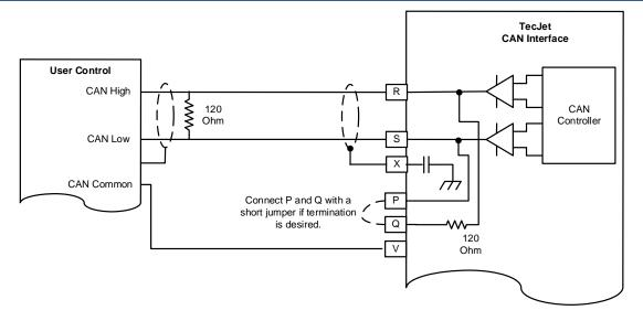
Figure 2-5. TecJet 85 CAN Wiring for Non-isolated Systems
