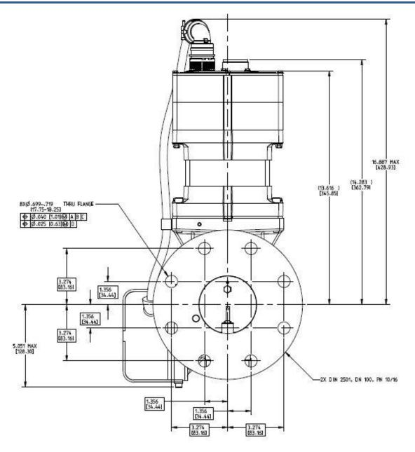
Figure 2-2d. Valve Inlet View
