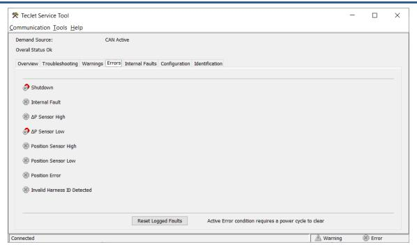
Figure 5-5b. Errors Screen after Power Cycle
