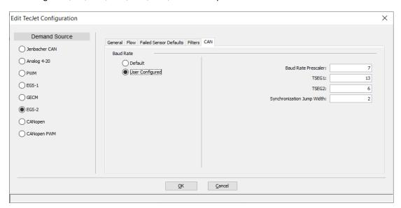
Figure 5-12b. Edit TecJet Configuration - CAN (User Configured)
