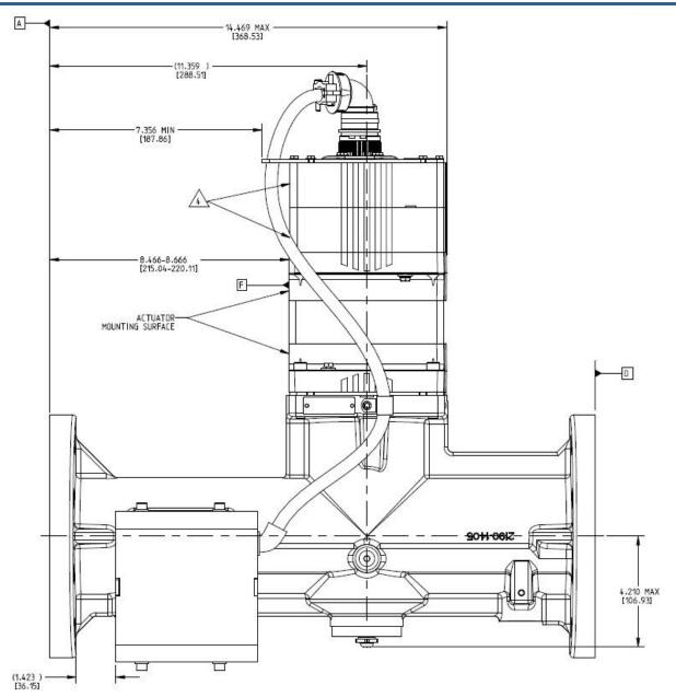
Figure 2-2c. Valve Outlet to Actuator Mounting View
