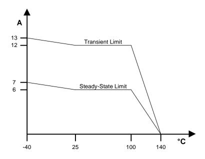
Figure 3-1. Current Limiting Based on Temperature
