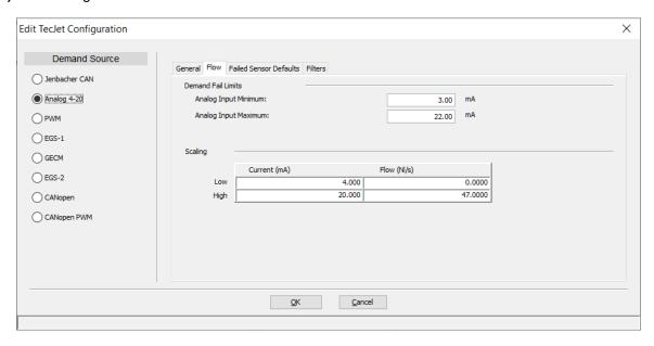
Figure 5-9b. Edit TecJet Configuration - Flow (Analog Demand)
