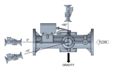
Figure 2-1c. Allowable Bore Orientations
