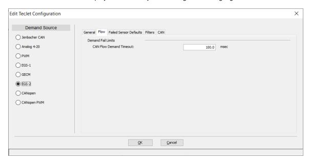
Figure 5-9a. Edit TecJet Configuration - Flow (CAN Demand)
