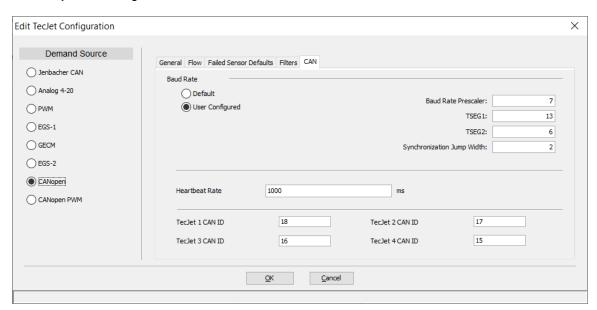
Figure 5-12c. Edit TecJet Configuration - CAN (User Configured)
