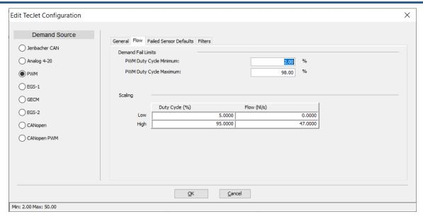
Figure 5-9c. Edit TecJet Configuration - Flow (PWM Demand)
