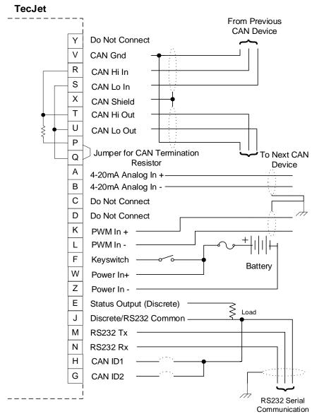
The recommended wire size for W and Z (Power Supply Inputs) is at least 1.3 mm² (16 AWG). For all other I/O, the recommended wire size is at least 0.5 mm² (20 AWG).
