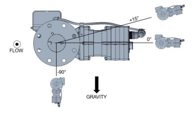
Figure 2-1b. Allowable Actuator Orientations
