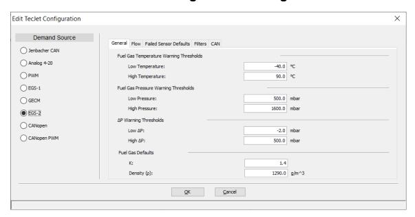
Figure 5-13. Load Configuration Settings
