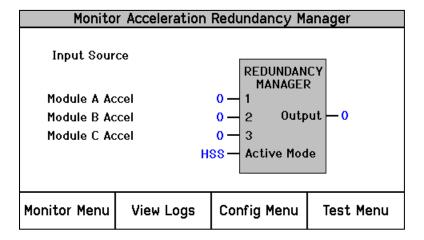
Figure 4-14. Acceleration Redundancy Manager
