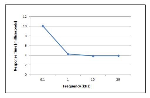
Figure 3-14. Total System Response Time Based on Sensed Frequency Level for Independent Trip Relay Models when Speed Redundancy Manager Function is not Configured
