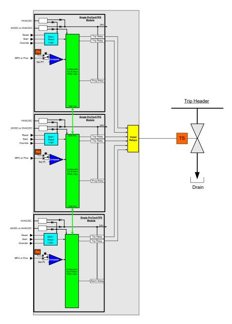
Figure 3-8. Simplex Trip Block Assembly
