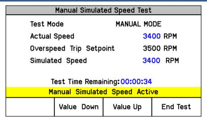
Figure 6-5. Manual Simulated Speed Test Screen
