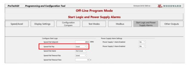
Figure 10-2. Speed Fail Trip Using PCT
