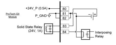
Figure 2-14f. Example Alarm Relay Wiring (External Supply)
