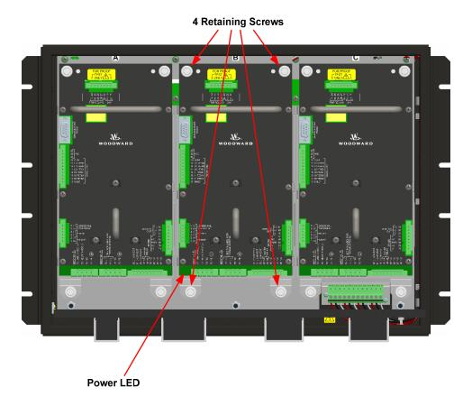
5. Remove module by pulling the two handles simultaneously.
