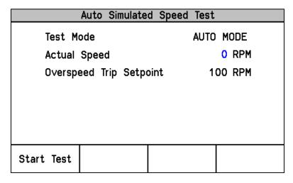
Figure 6-6. Auto Simulated Speed Test Screen
