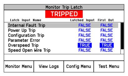
Figure 4-9. Monitor Trip Latch
