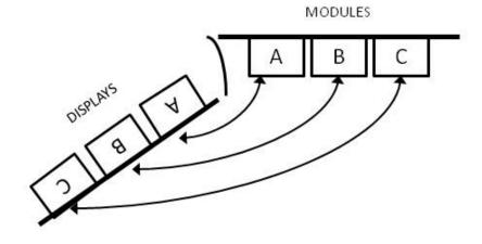
Figure 2-2b. Bulkhead Schematic Showing Front Panel A Connection to Module A and Front Panel C Connection to Module C—Top View
