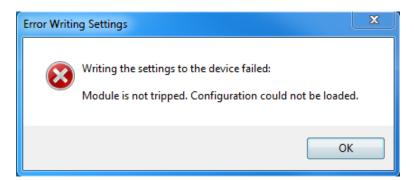
To load a configuration from a PC to a ProTech-GII, the ProTech-GII must be in a trip condition. If the unit is not in a trip condition, uploading is inhibited. If no trip condition is present, the configuration save will ask if a trip is desired. A trip will only be allowed if the other modules are not tripped.
