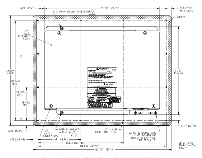
Figure 2-5a. Mounting Outline Diagram for Panel-Mount Models
