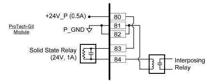
Figure 2-14e. Example Alarm Relay Wiring (Internal Supply)
