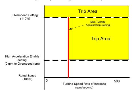
Figure 3-10. Over-Acceleration Enabling Diagram
