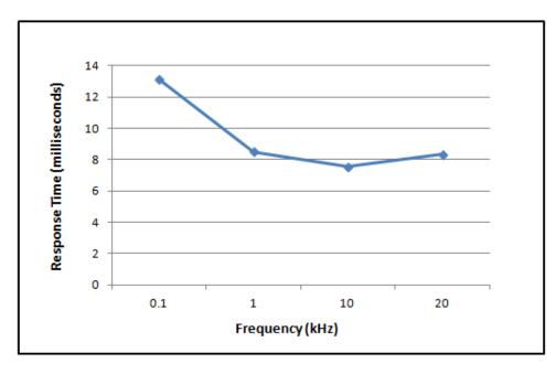
Figure 3-15. Total System Response Time Based on Sensed Frequency Level for Independent Trip Relay Models when Speed Redundancy Manager Function <u>is</u> Configured
