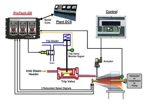
Figure 1-1. Typical ProTech-GII Application (Voted Trip Relay Models)
