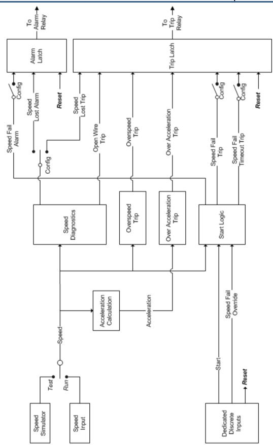
Figure 3-2. Module Diagram without Speed Redundancy Manager Configured
