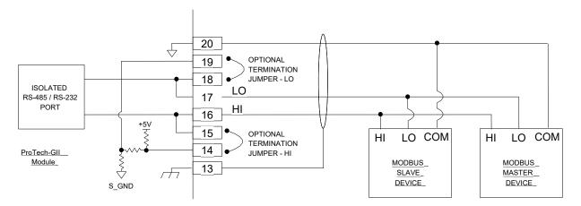
Figure 2-16b. Serial Com Port Interface Diagram—RS-485
