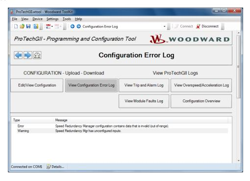
If a configuration error exists, the configuration is not saved and the following screen appears when trying to upload the settings file to the ProTech-GII.
