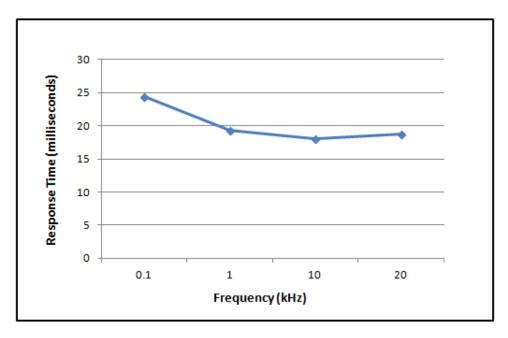
Figure 3-17. Total System Response Time Based on Sensed Frequency Level for 2003 Voted Trip Relay Models when Speed Redundancy Manager Function is Configured
