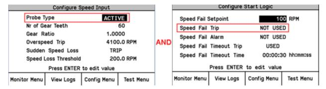
Figure 10-1. Configuration Guide - Front Panel Interface with Active Probe
