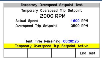
Figure 6-2b. Temporary Overspeed Test
