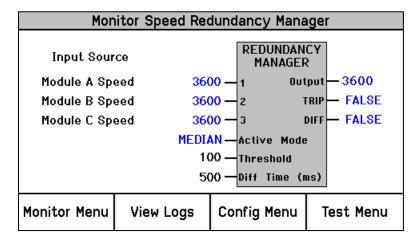
Figure 4-13. Speed Redundancy Manager
