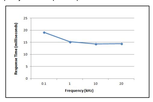
Figure 3-16. Total System Response Time Based on Sensed Frequency Level for 2003 Voted Trip Relay Models when Speed Redundancy Manager Function is <u>not</u> Configured
