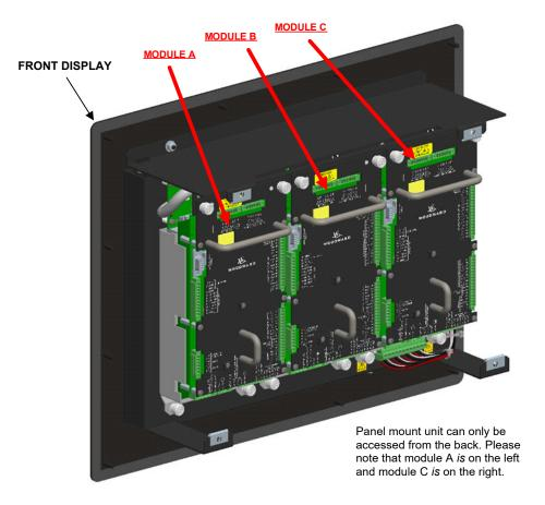
Figure 2-4c. Typical ProTech-GII Panel Mount Package—Rear View without Cover Showing Module Orientation
