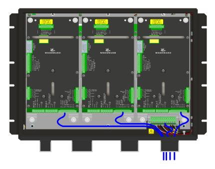
Figure 2-10c. Relay Output Field Wiring Routing & Stress Relief Diagram
