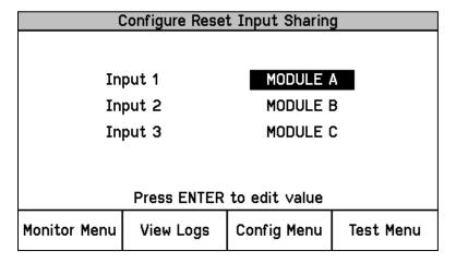
Figure 5-14. Configure Reset Input Sharing
