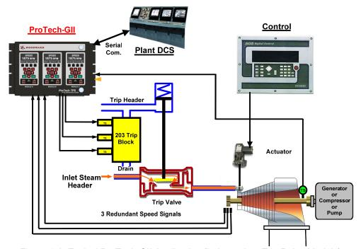
Figure 1-2. Typical ProTech-GII Application (Independent Trip Relay Models)
