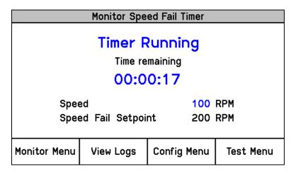
Figure 4-15. Monitor Speed Fail Timer
