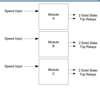
Figure 3-3. Basic Functional Overview of Independent Trip Relay Models
