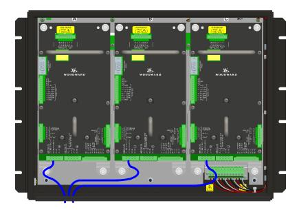
Figure 2-10a. Power Supply Field Wiring Routing & Stress Relief Diagram
