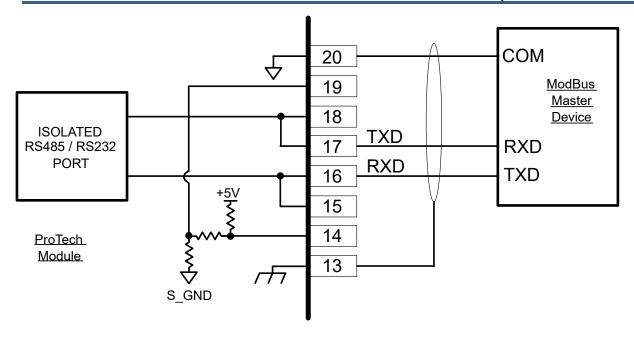
Figure 2-16a. Serial Port Interface Diagram—RS-232
