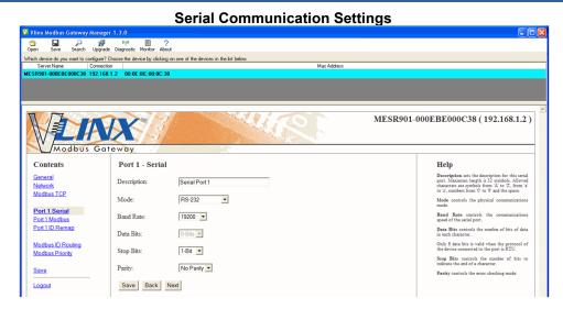
**Note:** For RS-485 communication, select RS-485 under Mode, and use the terminal block connections. The DB9 port is for RS-232 communications only.
