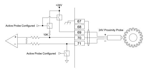
Figure 2-11b. Example Proximity Probe (Active Magnetic Pickup Unit) Wiring (Internal Power)
