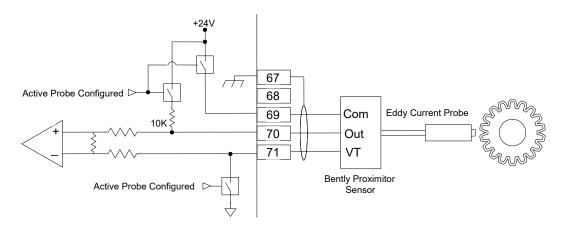
Figure 2-11d. Example Eddy Current Probe (Active Magnetic Pickup Unit) Wiring
