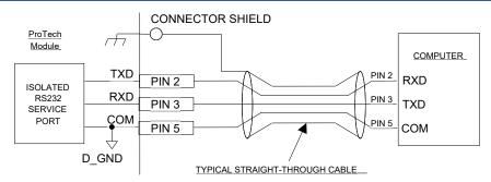
Figure 2-17. Programming and Configuration Tool Cable/Interface Diagram
