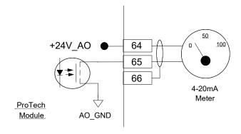
Figure 2-13. Example Analog Output Wiring
