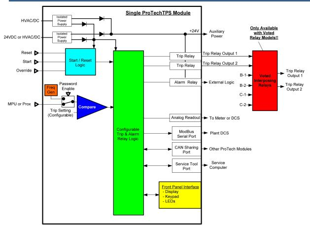
Figure 3-7. Functional Diagram of Single ProTech-GII Module with Voted Trip Relay Outputs
