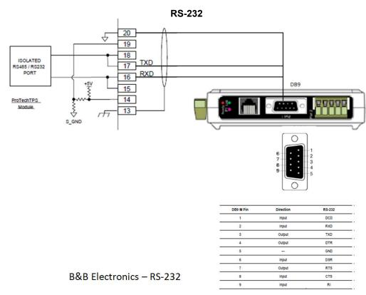
Note: The Serial DB9 connection is used for RS-232 communication only.
