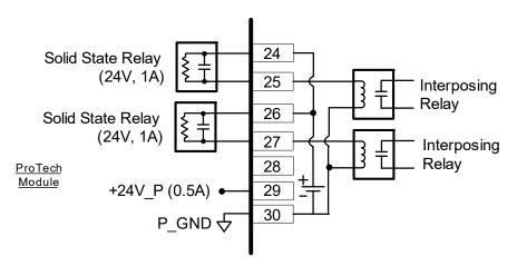
Figure 2-14c. Example Trip Relay Wiring (per Module) (Independent Trip Relay) (External Supply)
