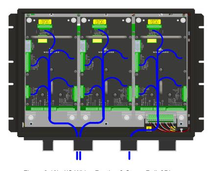
Figure 2-10b. I/O Wiring Routing & Stress Relief Diagram
