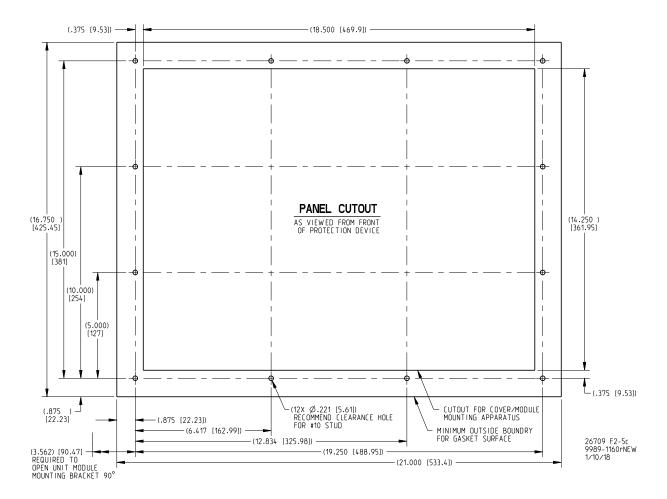
Figure 2-5c. Panel Cutout Diagram for Panel-Mount Models
