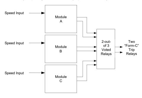
Figure 3-6. Basic Functional Overview of Voted Trip Relay Models
