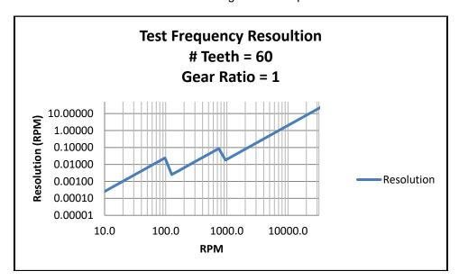
Figure 6-4. Test Frequency Resolution
