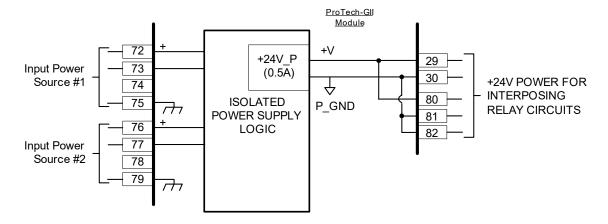
Figure 2-15. Power Supply Relationship Diagram
