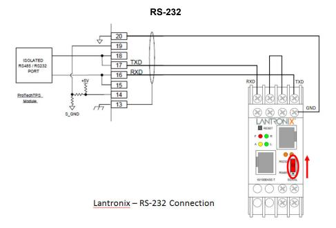
Verify that the dip switch on the front of the device is in the up position, indicating RS-232 communications.
