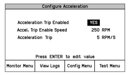
Figure 5-6. Configure Acceleration
