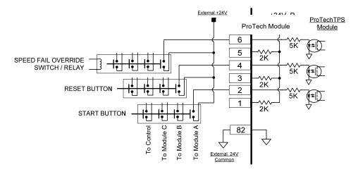
Figure 2-12b. Example Standard Discrete Input Wiring (External Power Option)
