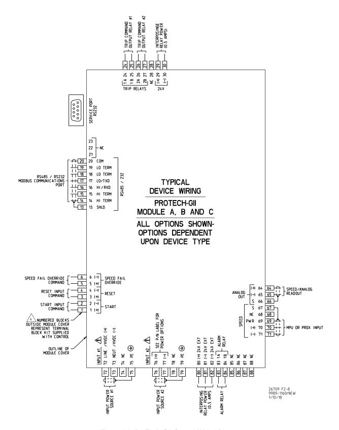
Figure 2-8. ProTech-GII Control Wiring Diagram
