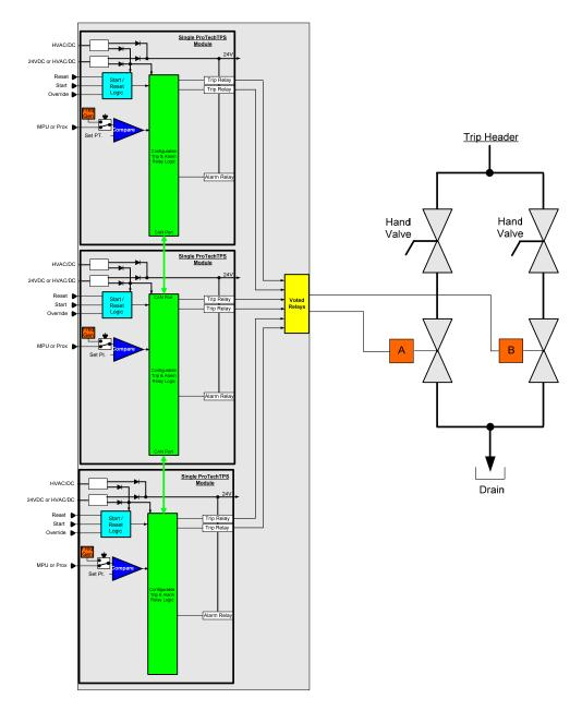
Figure 3-9. Dual Redundant Trip Block Assembly
