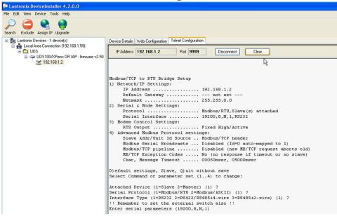
**Note:** For RS-485 communications, choose option 3 under interface type and don't forget to set the dip switch on the front of the device.
