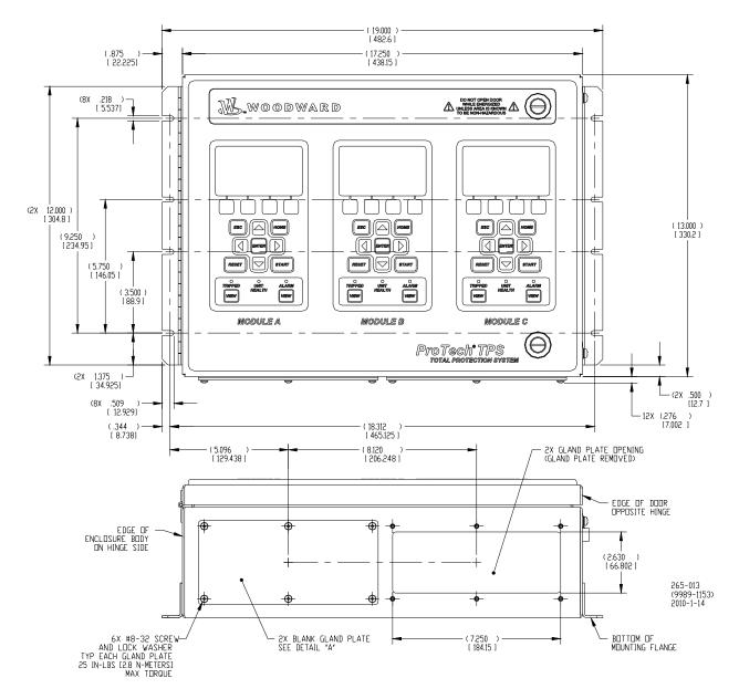
Figure 2-3. Mounting Outline Diagram for Bulkhead-Mounted Models
