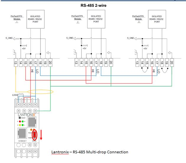
Verify that the dip switch on the front of the device is in the down position, indicating RS-485 communications. When configuring for RS-485, termination resistors (120  $\varsigma$ ) are needed at each end of the network. Note the location of the resistor on the device. The ProTech has the termination resistor built into the module, jumpers are necessary between terminals 14 – 15 and 18 – 19 to activate the termination.
