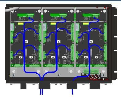
Figure 2-10b. Configurable I/O Wiring Routing & Stress Relief Diagram
