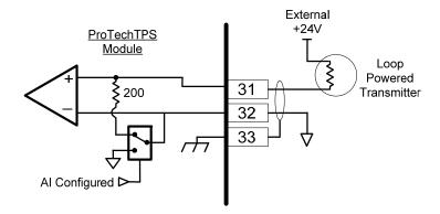
Figure 2-14. Example Configurable Input Wiring—Analog Input
