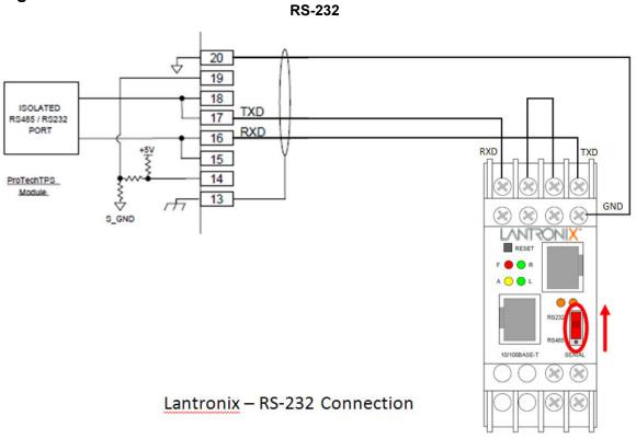
Verify that the dip switch on the front of the device is in the up position, indicating RS-232 communications.
