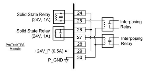
Figure 2-16b. Example Trip Relay Wiring (per Module) (Independent Trip Relay) (Internal Supply)
