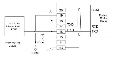
Figure 2-18a. Serial Port Interface Diagram—RS-232
