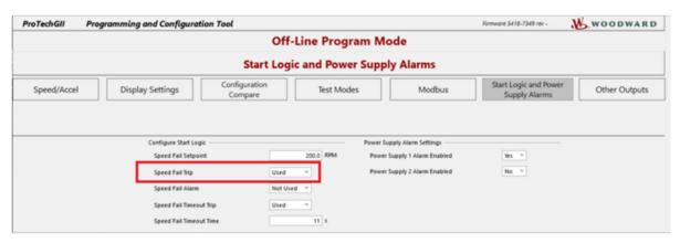
Figure 5-2. Speed Fail Trip Using PCT
