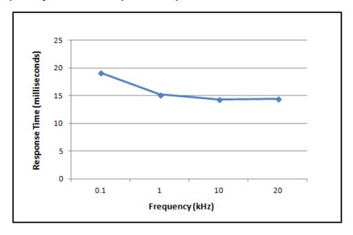
Figure 3-19. Total System Response Time Based on Sensed Frequency Level for 2003 Voted Trip Relay Models when Speed Redundancy Manager Function is <u>Not</u> Configured
