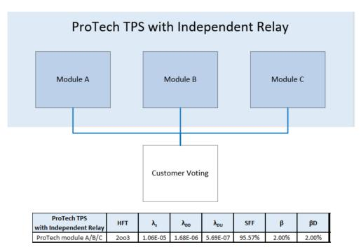
Figure 6-1. ProTech TPS with Independent Relay
