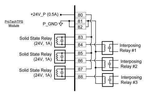
Figure 2-16e. Example Programmable Relay Wiring (Internal Supply)
