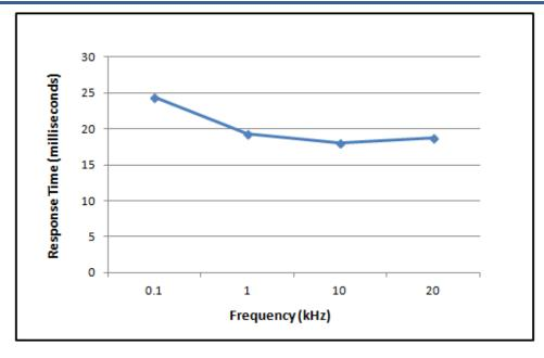
Figure 3-20. Total System Response Time Based on Sensed Frequency Level for 2003 Voted Trip Relay Models when Speed Redundancy Manager Function is Configured
