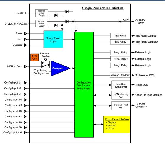
Figure 3-4. Functional Diagram of Single ProTech® TPS Module with Independent Trip Relay Outputs
