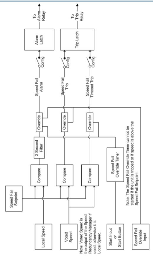
Figure 3-14. Start Logic Diagram
