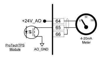
Figure 2-15. Example Analog Output Wiring
