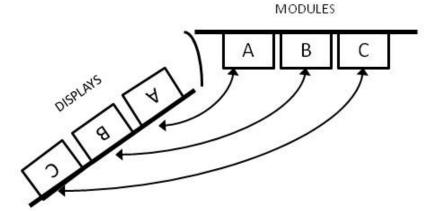
Figure 2-2b. Bulkhead Schematic Showing Front Panel A Connection to Module A and Front Panel C Connection to Module C—Top View
