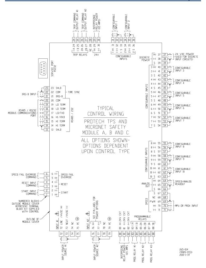
Figure 2-8. ProTech® TPS Control Wiring Diagram
