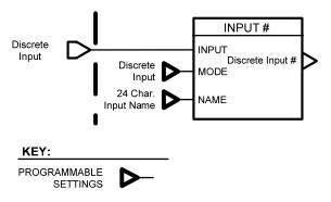
Figure 3-10. Discrete Input Example
