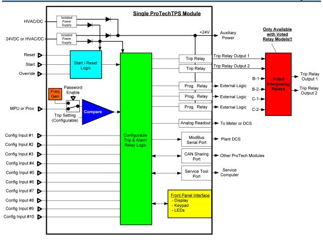
Figure 3-7. Functional Diagram of Single ProTech® TPS Module with Voted Trip Relay Outputs
