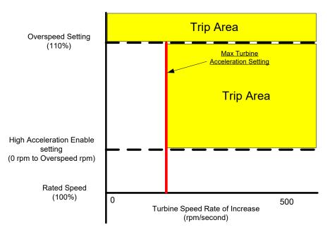
Figure 3-13. Over-Acceleration Enabling Diagram
