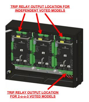
Figure 2-16a. Example Trip Relay Output Wiring
