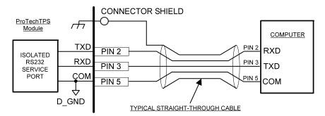
Figure 2-19. Service Tool Cable/Interface Diagram
