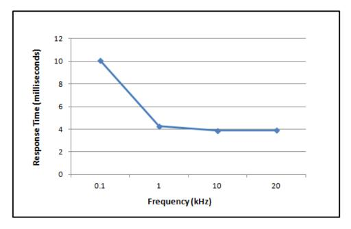
Figure 3-17. Total System Response Time Based on Sensed Frequency Level for Independent Trip Relay Models when Speed Redundancy Manager Function is Not Configured
