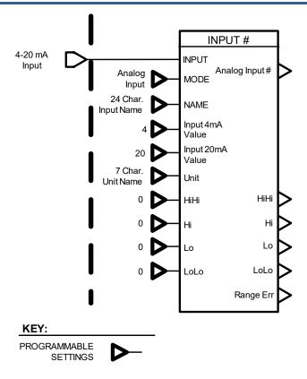
Figure 3-11. Analog Input Example
