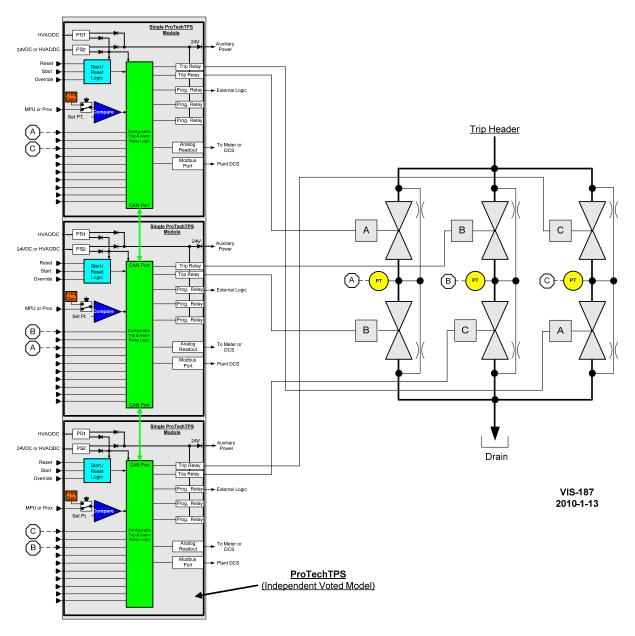
Figure 3-5. Example TMR Trip Block Assembly Interface
