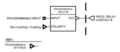
Figure 3-12. Programmable Relay Output Diagram
