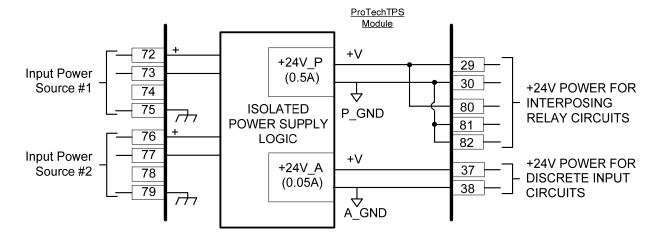
Figure 2-17. Power Supply Relationship Diagram
