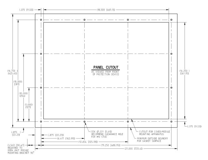
Figure 2-5c. Panel Cutout Diagram for Panel-Mount Models
