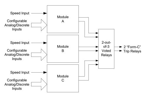
Figure 3-6. Basic Functional Overview of Voted Trip Relay Models
