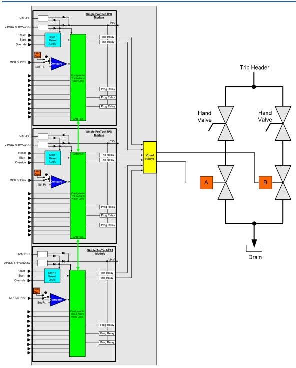
Figure 3-9. Dual Redundant Trip Block Assembly
