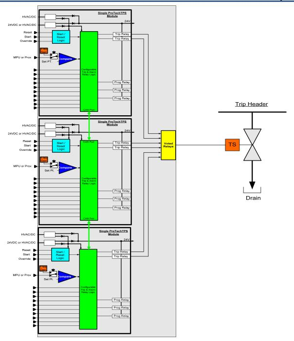
Figure 3-8. Simplex Trip Block Assembly
