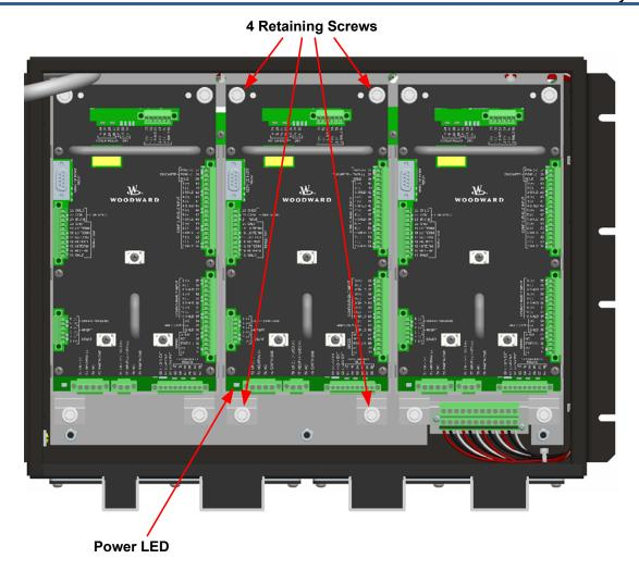
5. Remove module by pulling the two handles simultaneously.
