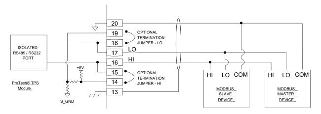
Figure 2-18b. Serial Com Port Interface Diagram—RS-485
