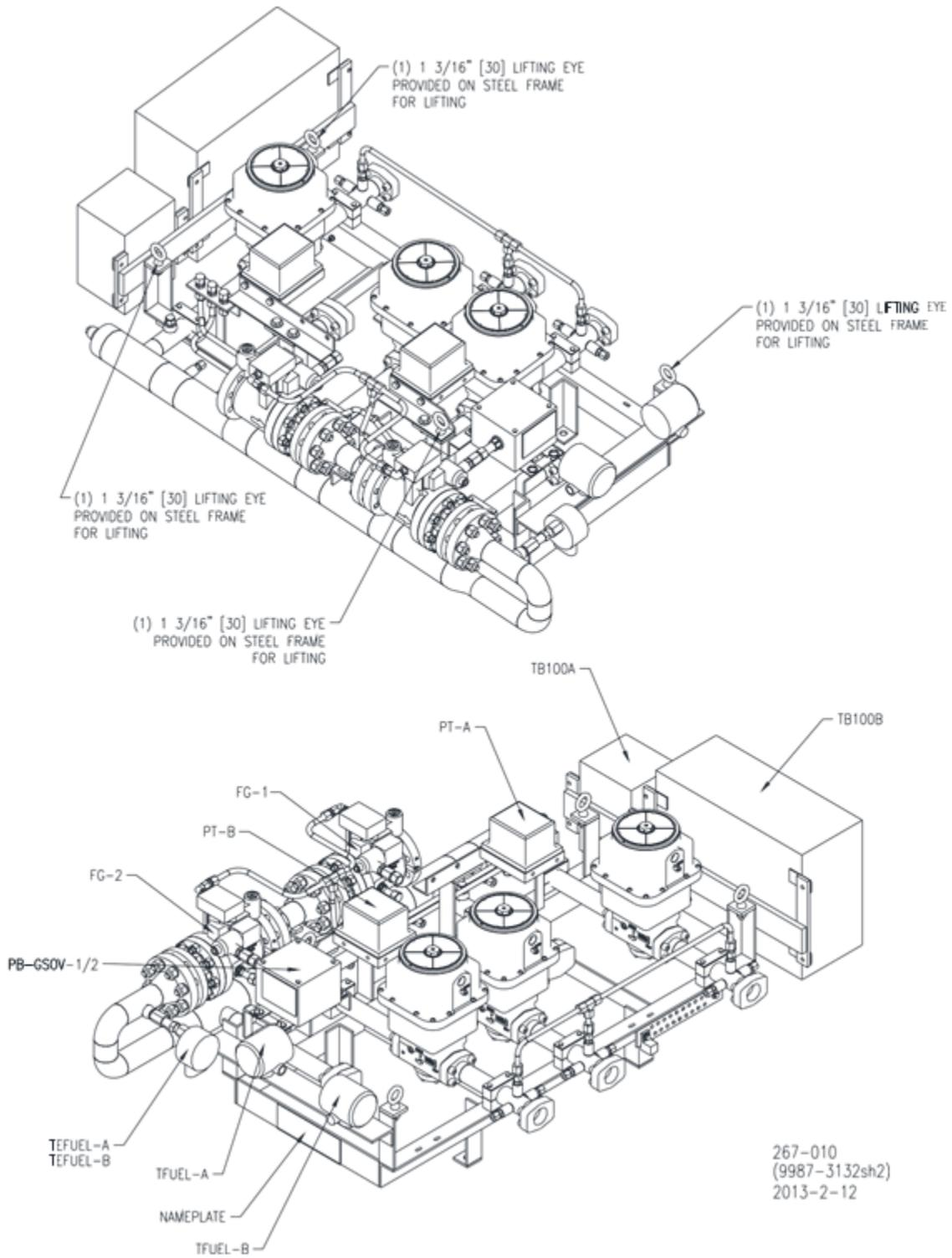
Figure 2-2c. Standard Woodward GS6 Gas Fuel Skid PGT25+ DLE & LM2500+ DLE
