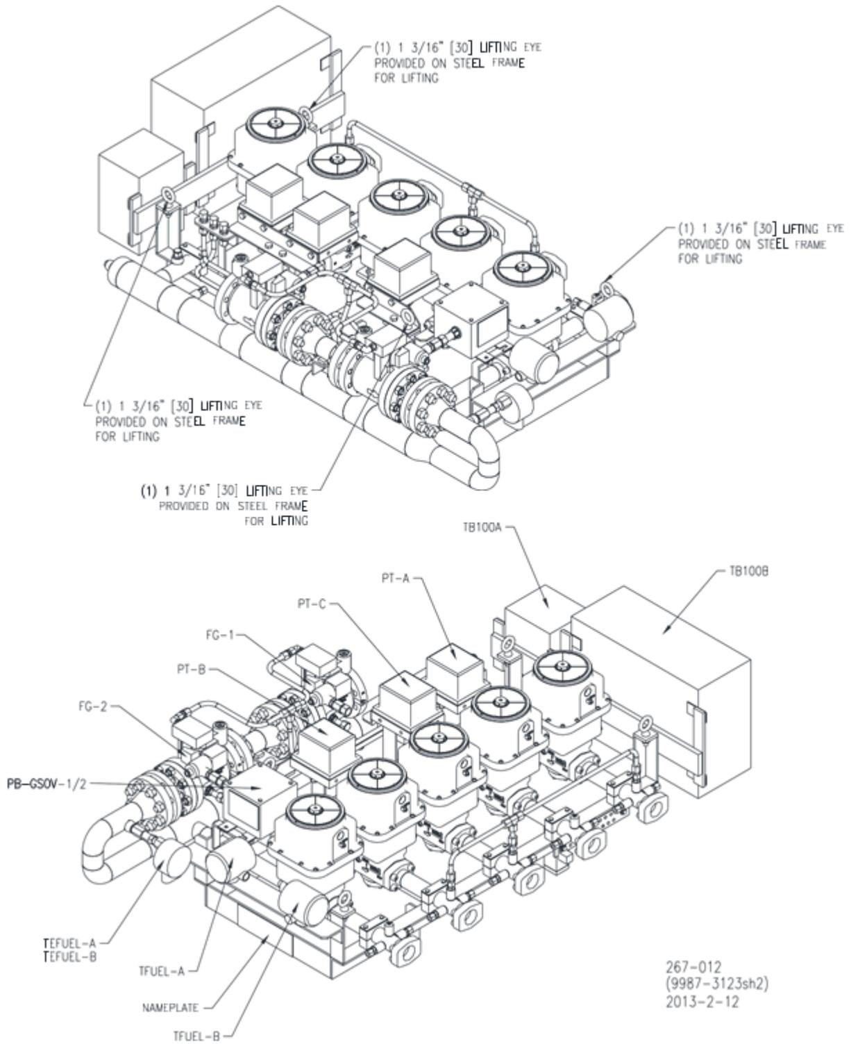
Figure 2-3c. Standard Woodward GS6 Gas Fuel Skid PGT25+ G4 DLE & LM2500+ G4 DLE
