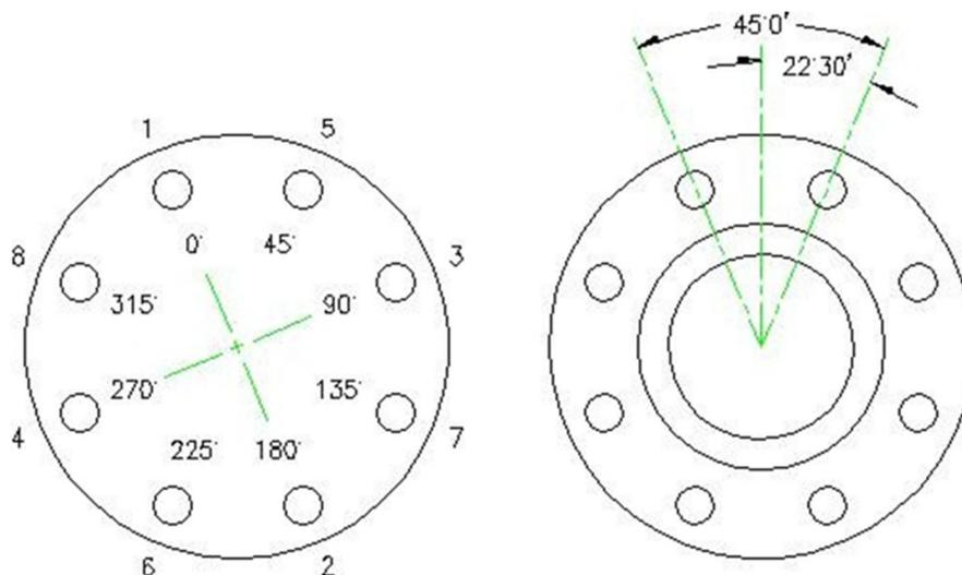
Figure 2-1. Bolt Tightening Sequence
