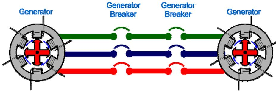
The voltage amplitudes (controlled by the voltage regulator) of the systems must be closely matched (usually between 1-5 %) before the generator breaker is closed. If they are not closely matched, the generator could produce large amounts of Reactive Power:
