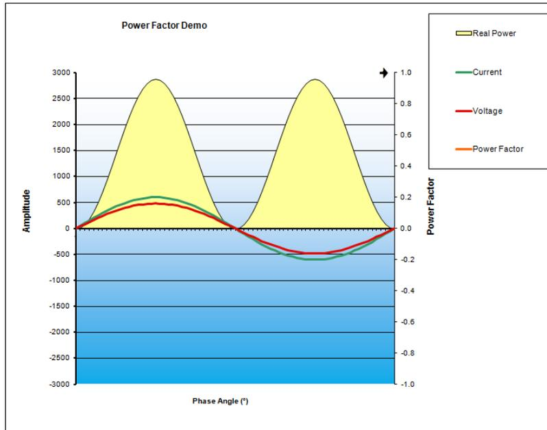
Notice that the voltage (green line) and current (red line) cross the zero reference at the exact same time. If you multiply the voltage and the current together, you get the real power curve, which is always positive. Multiplying two negative numbers together is a positive number. The average of this curve is the average power. The phase difference between the voltage and current is zero. Cosine of zero = 1.0 which is Unity Power Factor.
