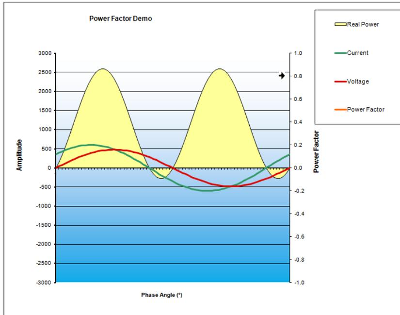
Notice that current leads the voltage by a specific number of degrees. The same reactive current can be seen. This condition is not seen very often as most Power Factors are lagging and not leading, like this is shown.
