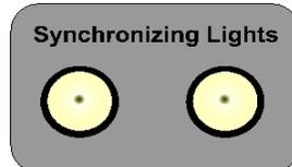
These usually consisted of two or three light bulbs across one phase or across all phases, on the generator. When the phase of both generators were 180 degrees out of phase, the light bulbs were on bright. As the phases of the generators got closer and closer, the voltage across the light bulbs became less and less. Until the phases were directly on top of each other, when the voltage between the two are close to zero.
