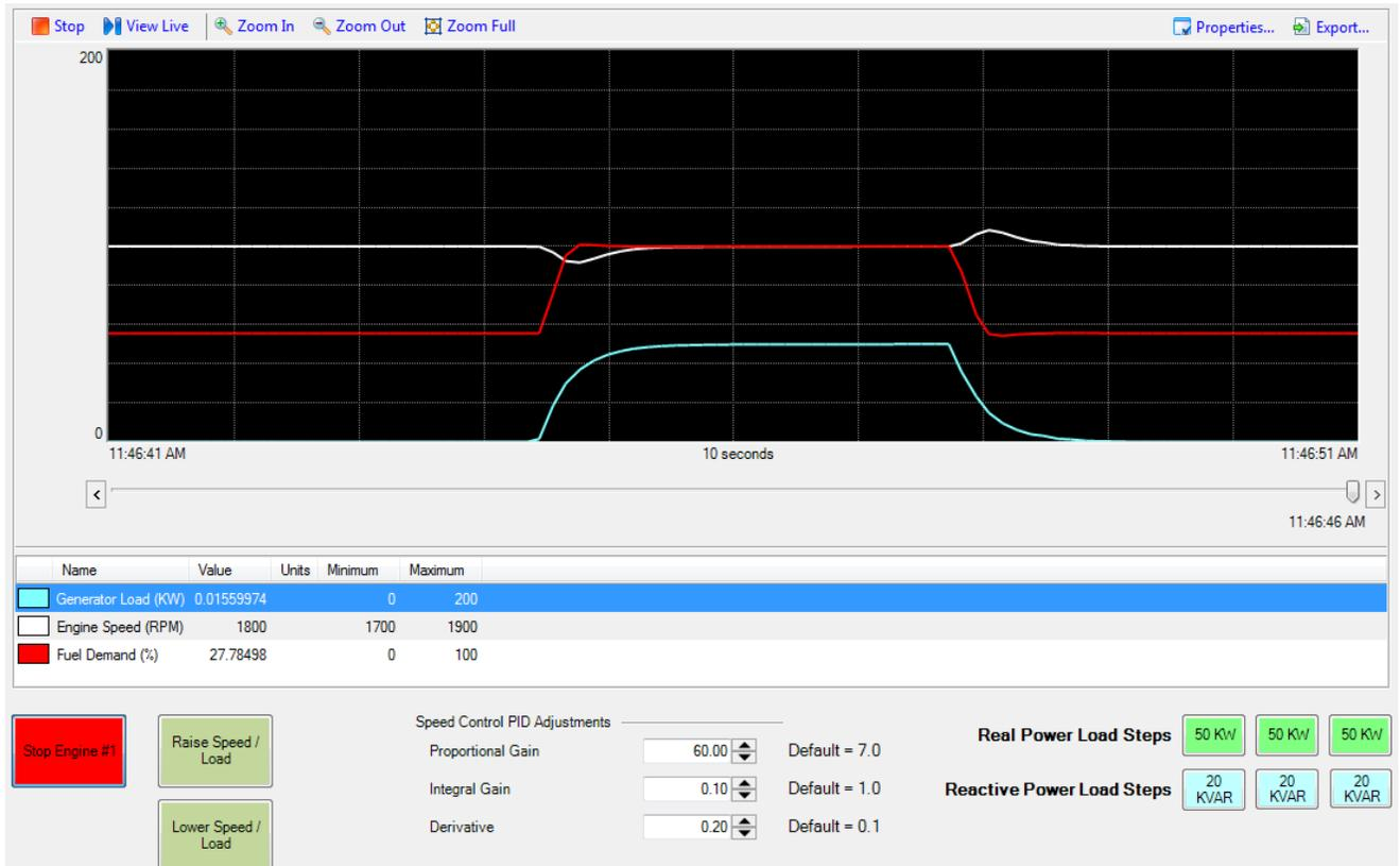
Put the Speed Control PID Adjustments back to the default values when done. Proportional Gain = 7.0, Integral Gain = 1.0, and Derivative = 0.1. Stop all of the engines and open all of the breakers.
