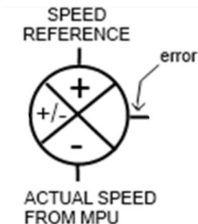
The summing point is where all signals in a control loop add up and must equal zero to allow the electronic control to be controlling the engine at a steady state condition. The advantage of a summing point is that many parameters, in addition to speed, can be sensed and sent to a summing point and controlled at a desired set point. A few examples are speed, pressure, temperature, kW power, and fuel demand limiting.
