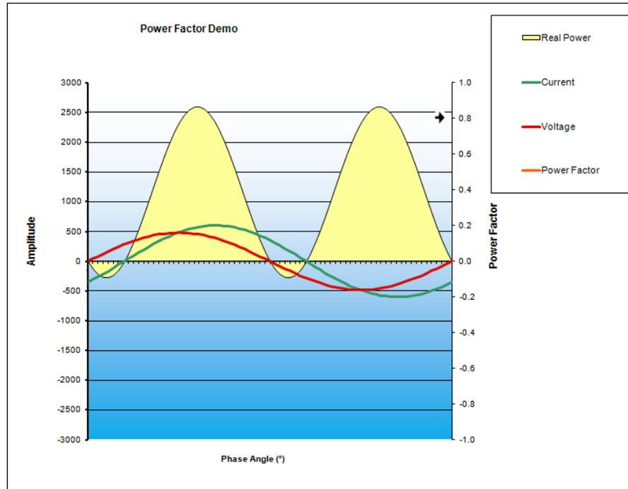
Notice that the voltage leads the current by a specific number of degrees. Also notice that there is a certain amount of power that is below zero (yellow curve below zero). This is the Reactive Power component. This chart shows the phase difference between the voltage and the current at about a 0.8 Power Factor.
