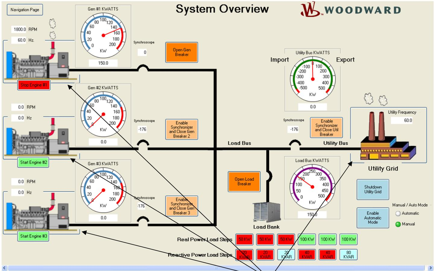
Each engine and the Utility Grid (Mains) is a **HOT BUTTON**. Clicking on each of the engine icons or the Utility Grid (Mains) icon will allow you to navigate to these pages.
