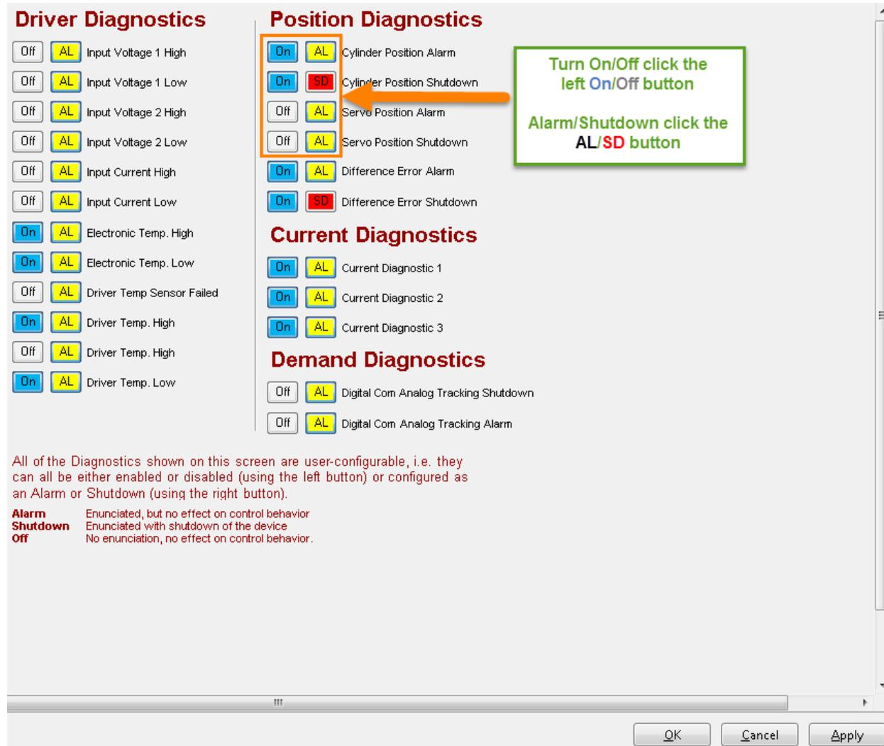
Figure 6-56. Process Fault and Status Flag Configuration Page
