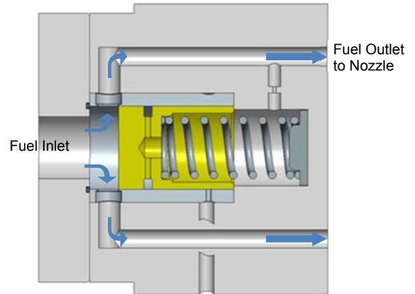
Figure 1-1b. FDV with Piston in Open Position
