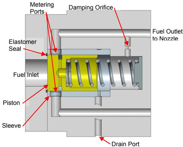
Figure 1-1a. FDV with Piston in Closed Position
