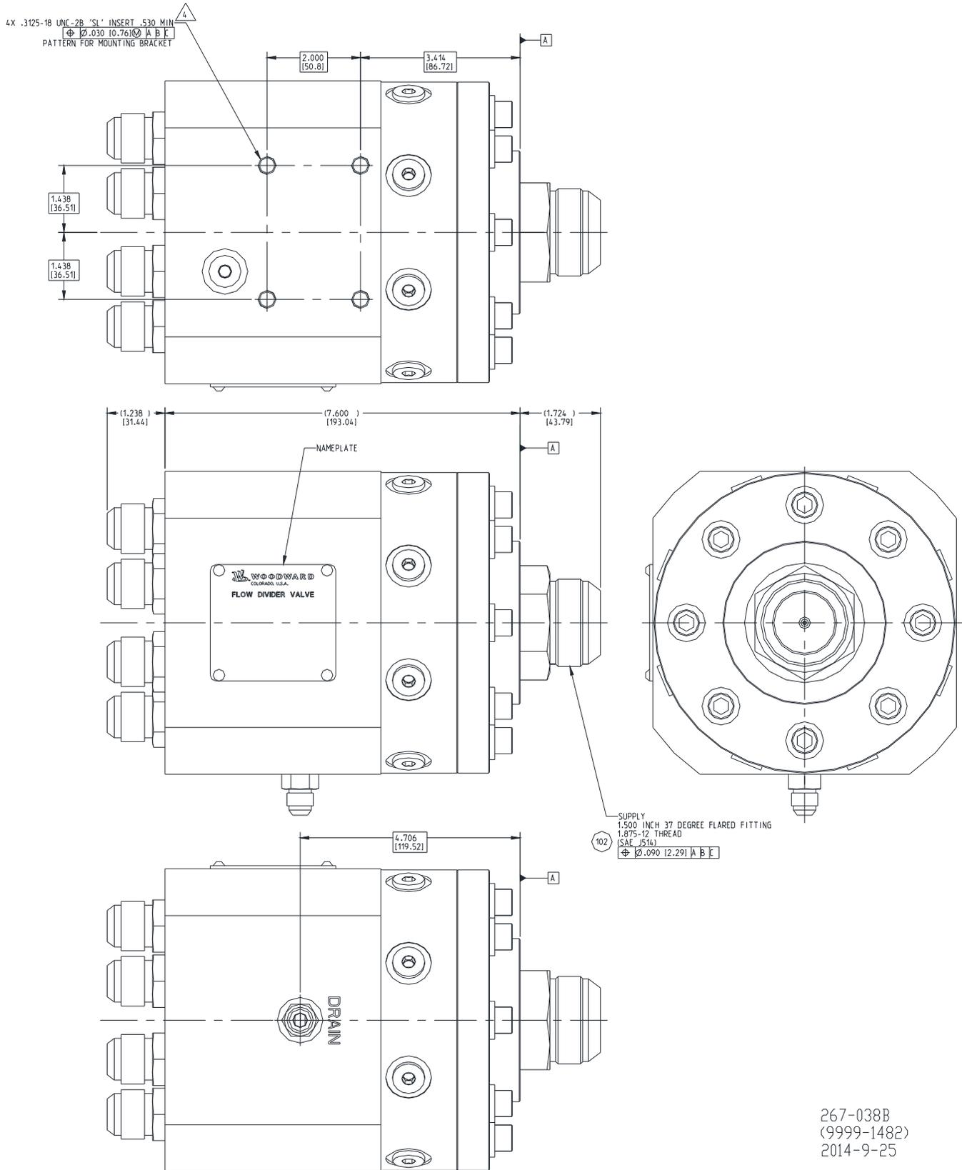
Figure 1-2b. Installation Diagram
