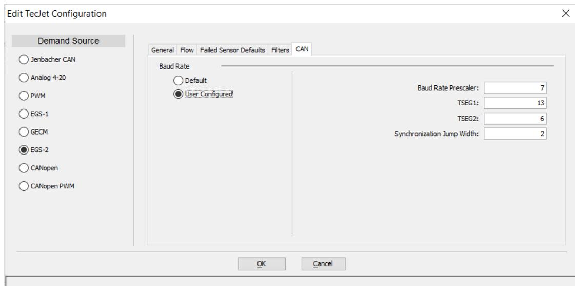
Figure 5-12b. Edit TecJet Configuration - CAN (User Configured)
