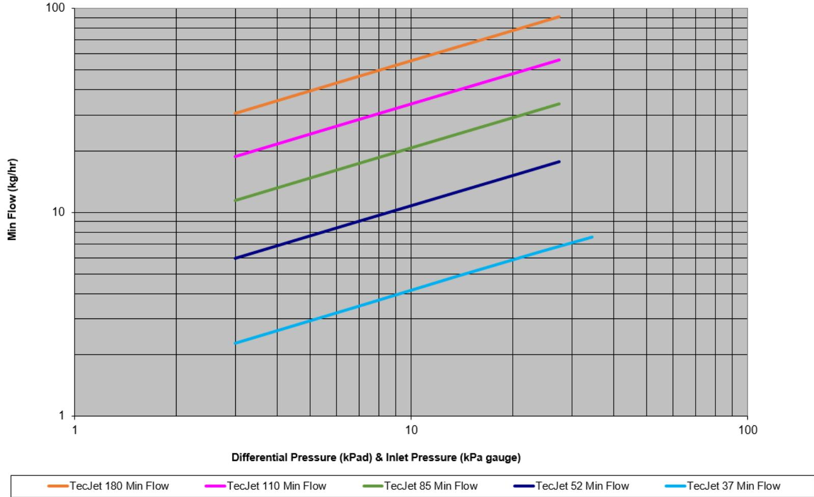
Figure 4-4. Minimum Natural Gas Flow Capacity of TecJet 180, 110, 85, 52 and 37 (Natural Gas, SG=0.6, Sea Level)
