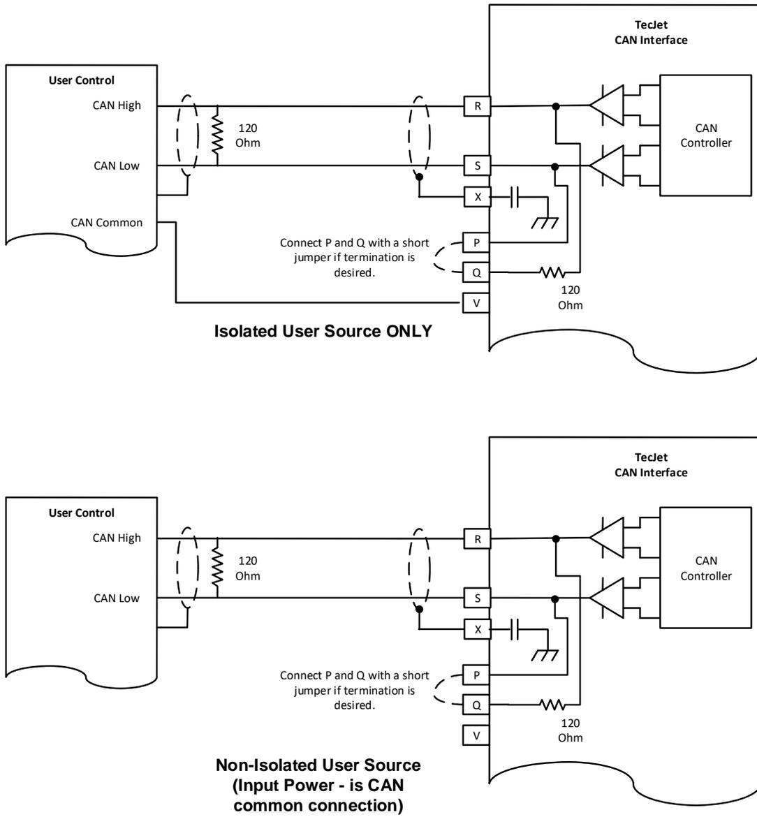
Figure 2-7. TecJet 52 CAN Wiring for Isolated/Non-Isolated Systems
