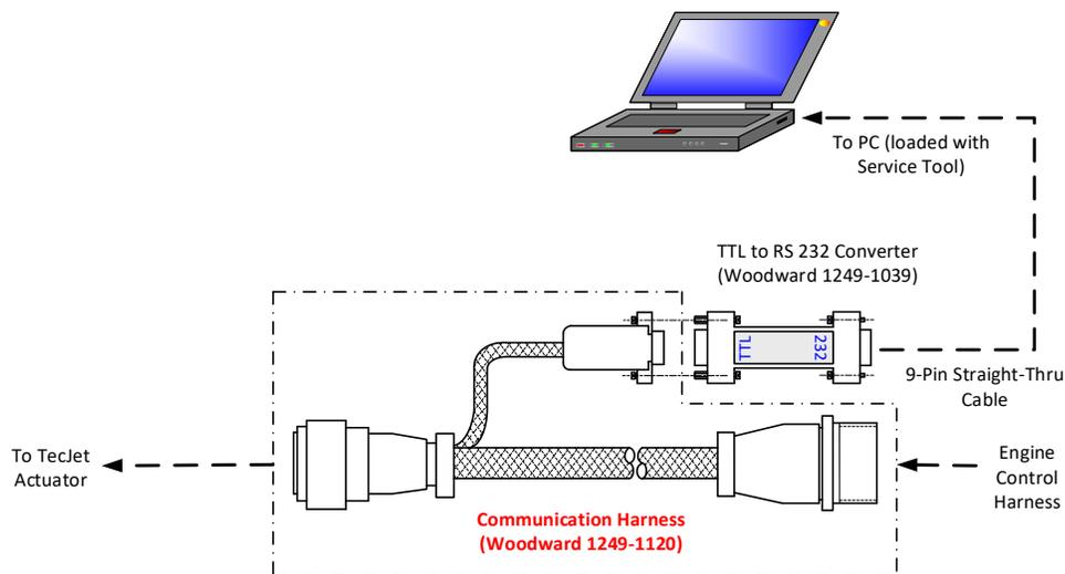
Figure 5-1. Communication- Harness Connections
