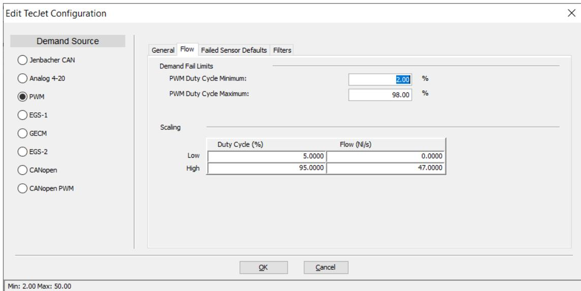
Figure 5-9c. Edit TecJet Configuration - Flow (PWM Demand)
