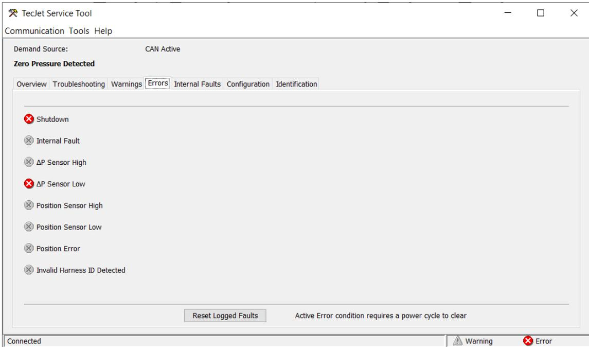
Figure 5-5a. Errors Screen before Power Cycle
