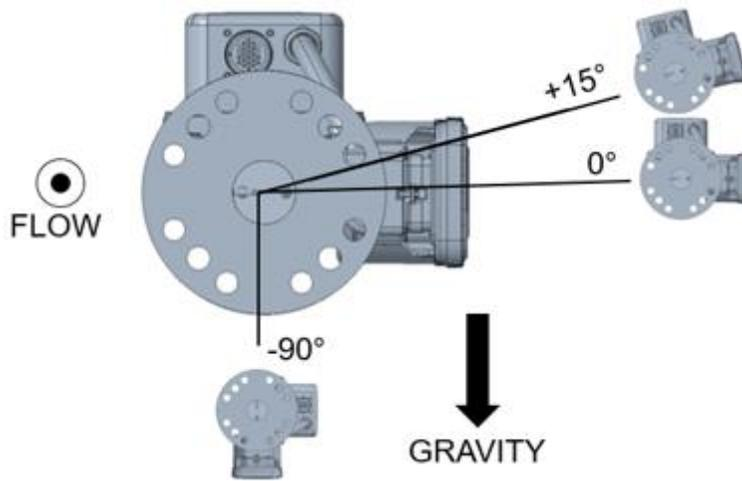
Figure 2-1b. Allowable Actuator Orientations
