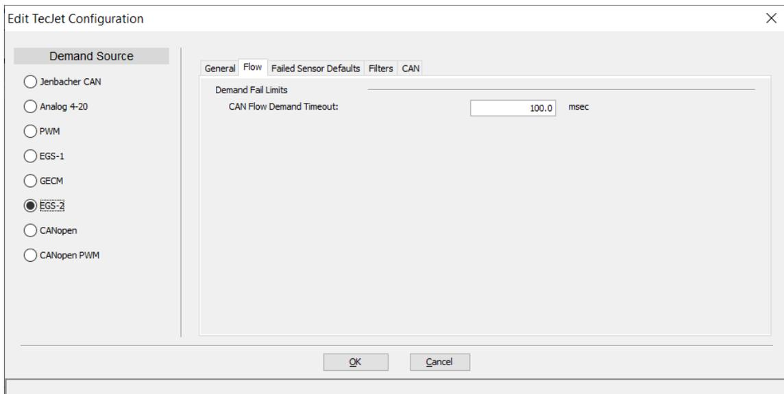
Figure 5-9a. Edit TecJet Configuration - Flow (CAN Demand)
