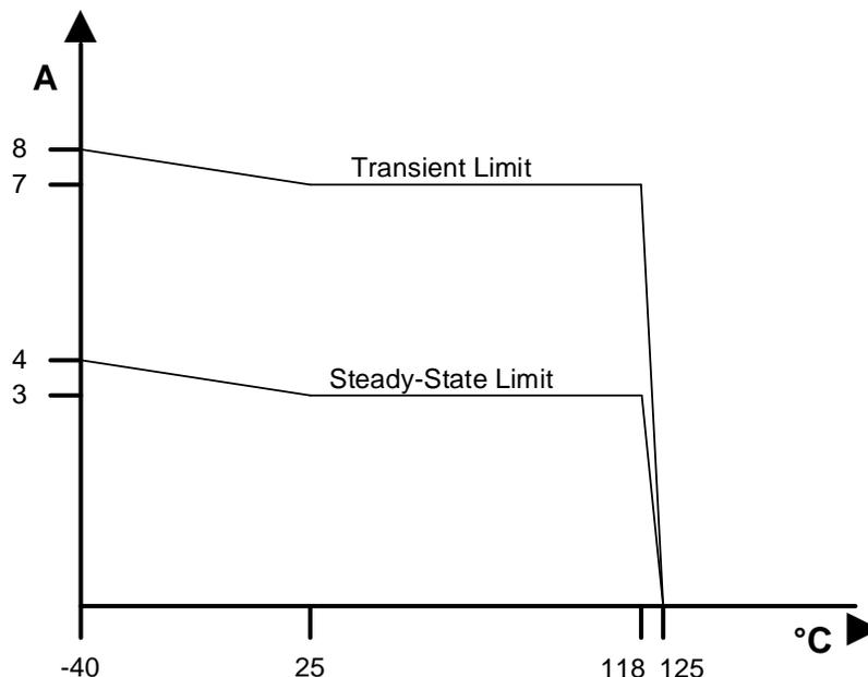
Figure 3-1. Current Limiting Based on Temperature
