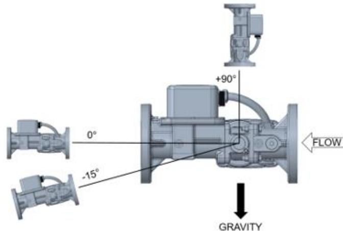
Figure 2-1c. Allowable Bore Orientations
