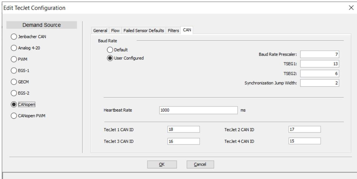
Figure 5-12c. Edit TecJet Configuration - CAN (User Configured)
