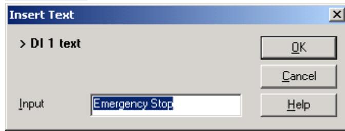
**Input Relay** The first line of text is the parameter description. Below the parameter description is the input field. The relay manager function linking is configured here. The numeric codes for the desired functions are linked with the logic symbols listed below. Up to three functions may be linked. The links are transmitted in three sequential words. The numeric codes for the relay manager functions may be found in the product manual that is being configured.
