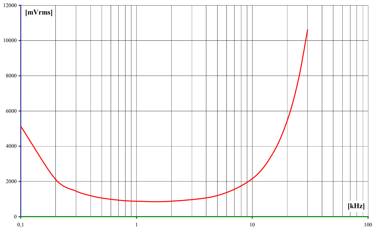
Figure 5-21: Minimal necessary input voltage depending on frequency
