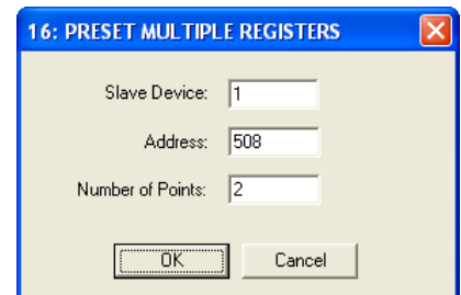
Figure 3-7: Modbus - configuration example 4 - active power
