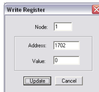
Figure 3-37: Modbus - write register - resetting the default values
