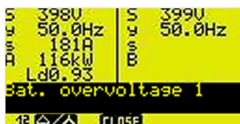
Fig. 104: LS-5x1 Main screen (example)
