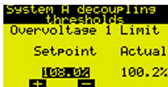
Fig. 120: For decoupling valid / not valid (example)
