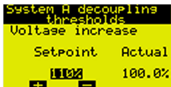
Fig. 122: Decoupling voltage increase (example)
