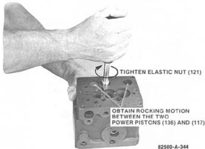
Figure 4-1. Obtaining Rocking Motion in Power Pistons
