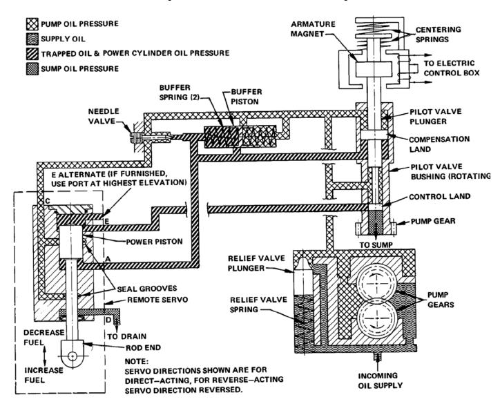
Figure 1-5. Schematic Diagram for EG-R Actuator
