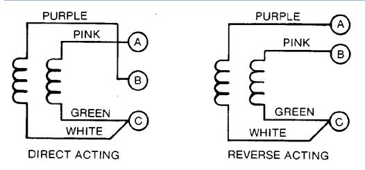
Figure 1-8. EG-3C and EG-R Wiring Diagrams
