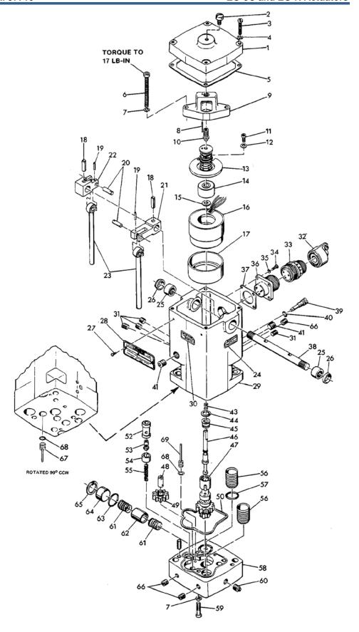
Figure 4-1. Exploded View, EG-3C Hydraulic Actuator
