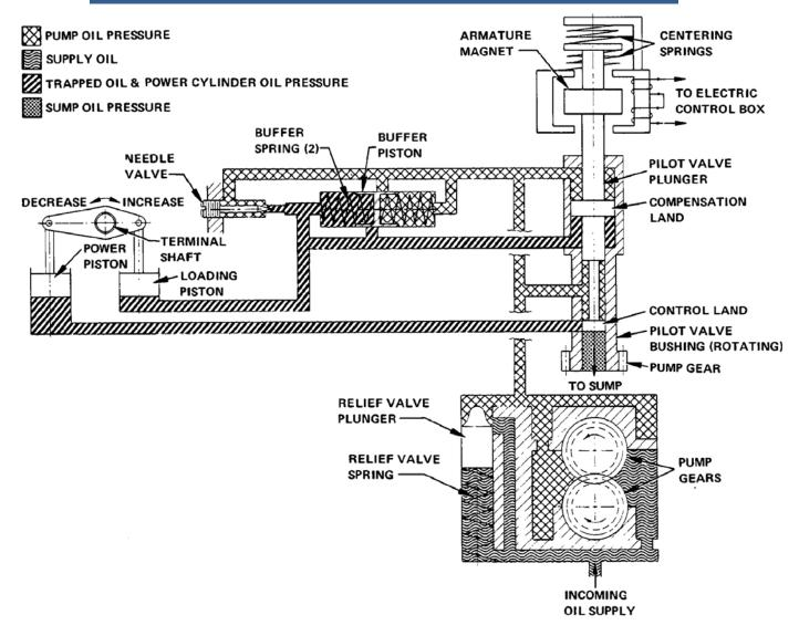
Figure 1-4. Schematic Diagram of EG-3C Actuator
