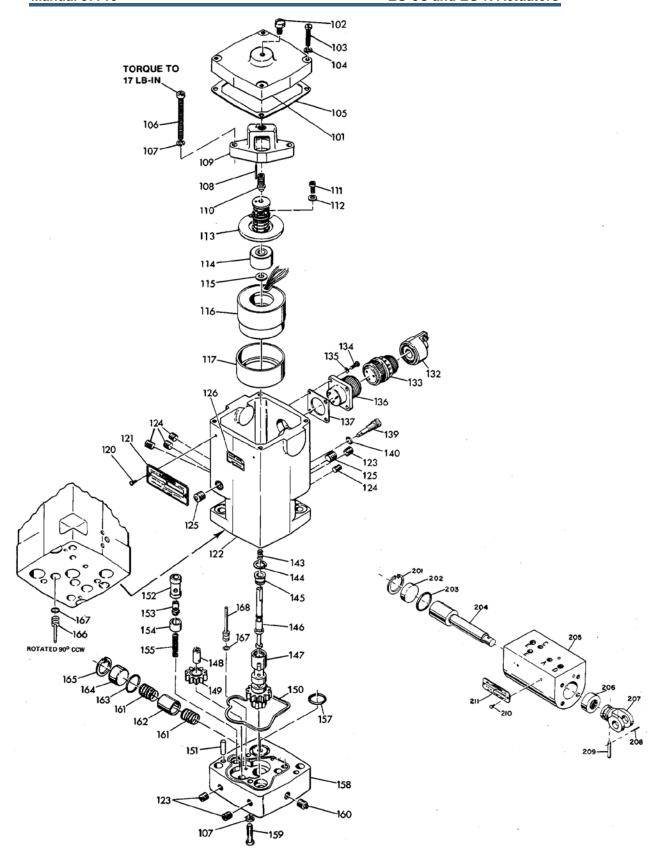
Figure 4-2. Exploded View, EG-R Hydraulic Actuator
