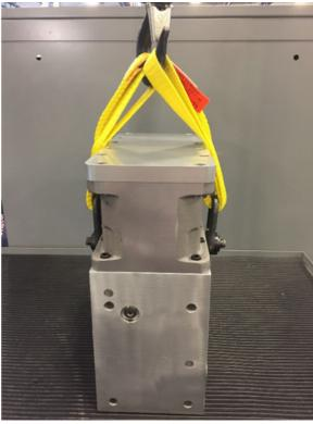
Figure 2-1. Lifting Sling Installation
