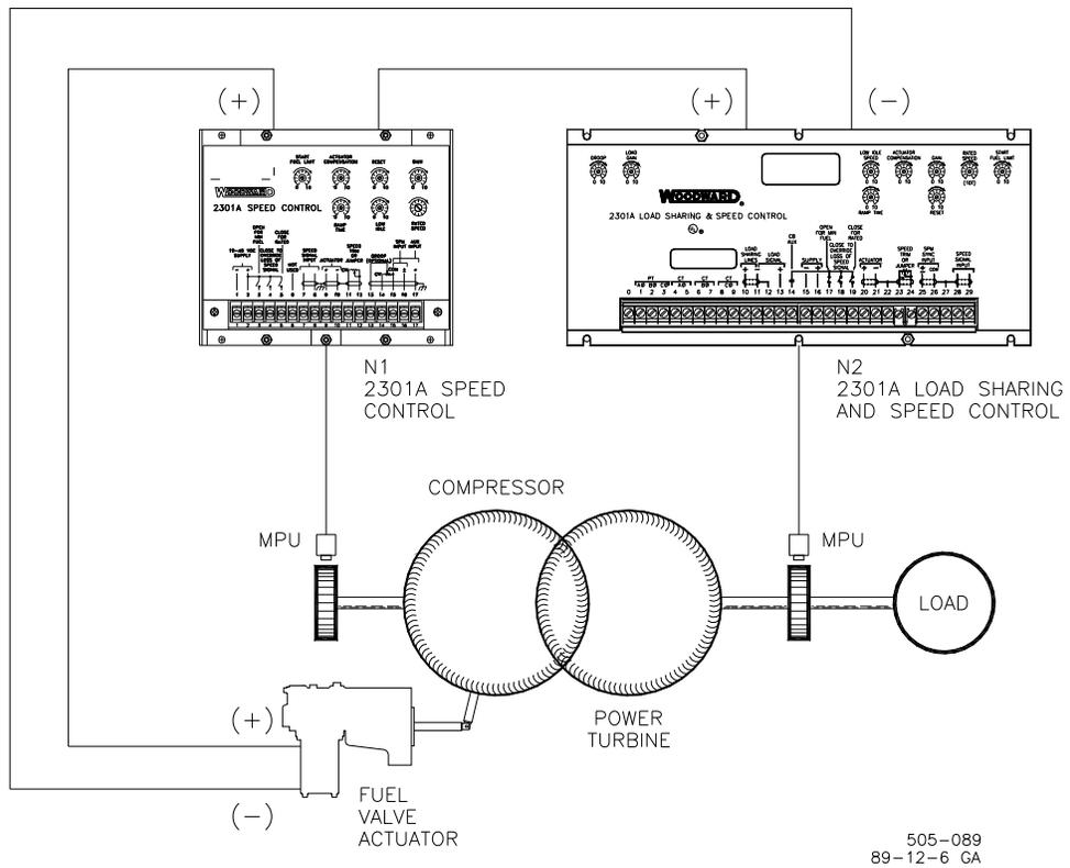
Figure 1-2. Block Diagram of Load Sharing and Speed Control Application
