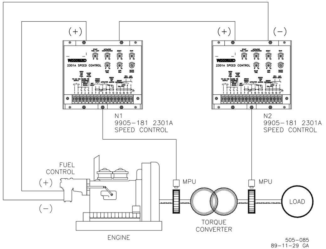
Figure 1-1. Block Diagram of Speed Control Application
