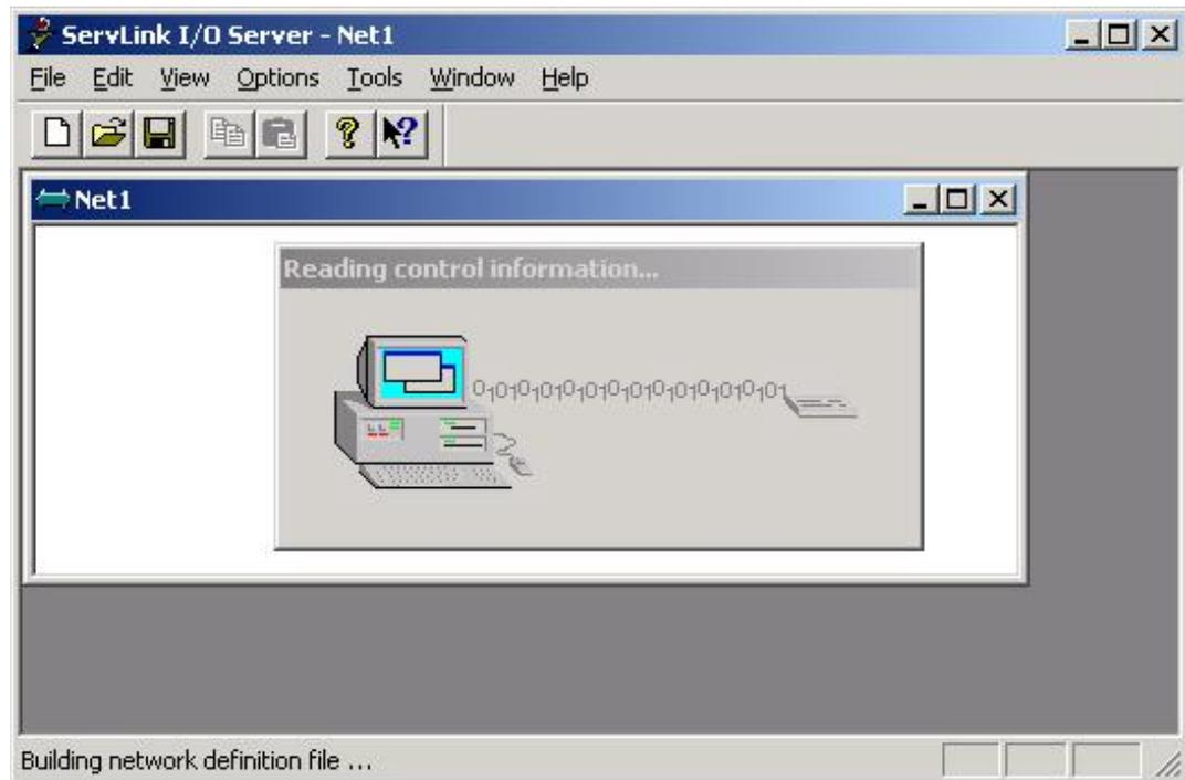
Once communications are established, and the data is read from the control network, the ServLink software will show each control it is communicating on the network by that control's network address. Here is a typical ServLink network definition screen for an EGCP-3.
