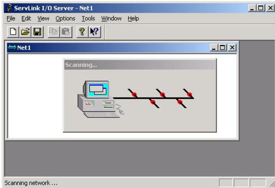
When communications are established with the control network, the scanning screen will change to display that the ServLink software is reading the control information. That screen will look like this:
