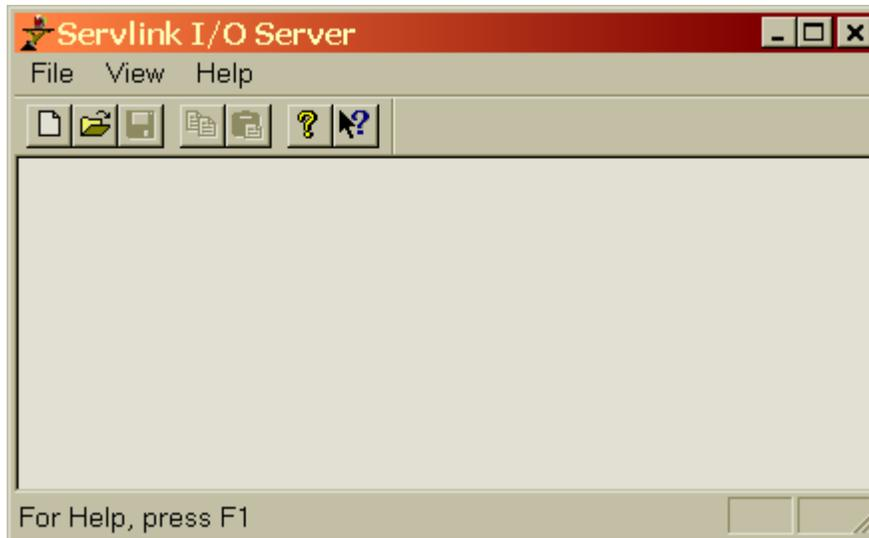
The first action to take inside the ServLink screen is to set up a new network definition file. Click once on **F**ile, and then on **N**ew as shown. The new network definition window will pop up on the computer screen.
