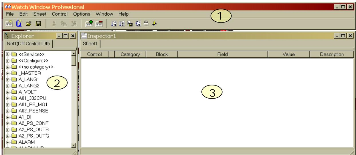
The Application Control window (1) is the main window for the software. It is used to manage the Explorer window (2) and the Inspector window (3). A tool bar is provided with icons to Open, close, and save Inspectors, and to upload and download the tunable setpoints.
