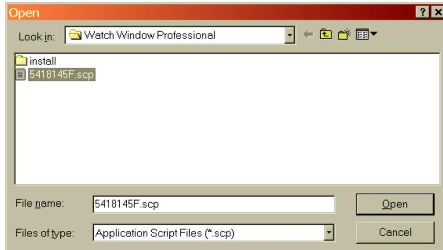
After the Open button is pressed a warning box will appear that tells the user that the control inputs and outputs will be locked during the download. Hit the Yes button to continue. Then a status bar will appear updating the file transfer progress.
