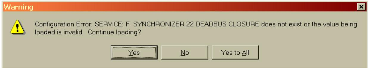
Depending on which revision was originally in the control, there may be several of these variables that can not be found. They can be verified one at a time by clicking the Yes button or all of them can be verified by clicking the Yes to All button. When the transfer is complete click on the Yes button to reset the control. Setpoint files can only be transferred when the unit is shut down.
