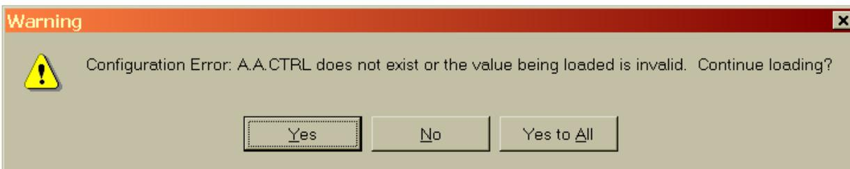
These configuration errors are the result of software changes in the control. The variables that were saved in the setpoint file of the previous version either no longer exist or have a different name in the new revision. Most of these are not important, however a few may be. For example the Deadbus Closure setting from the Synchronizer menu.
