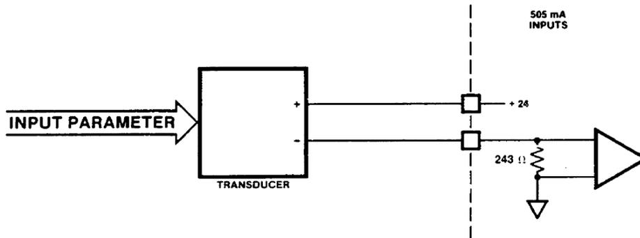
Figure 2-5. Two-Wire Transducer System
