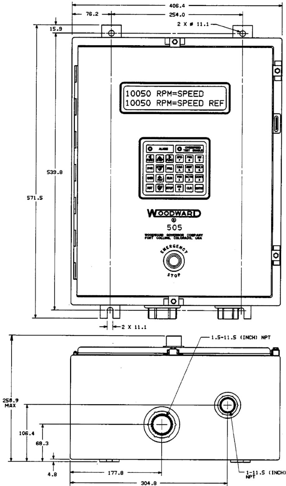
Figure 1-1a. 505 Control Layout (standard enclosure)
