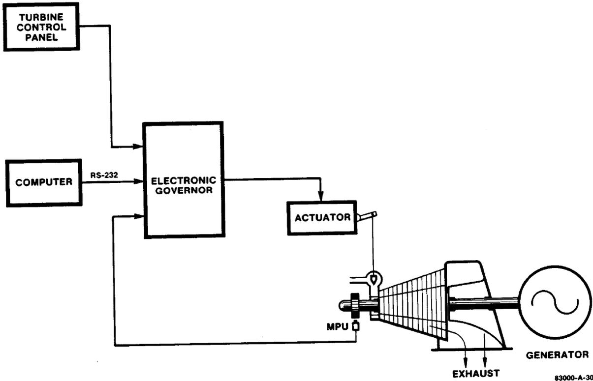
Figure 2-4. 505 Communication through an RS-232 Line
