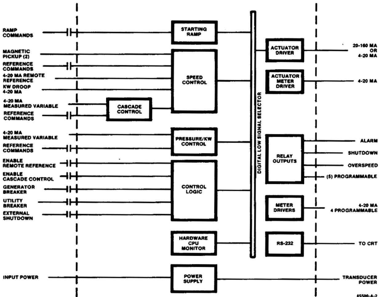
Figure 2-1. Simplified 505 Block Diagram
