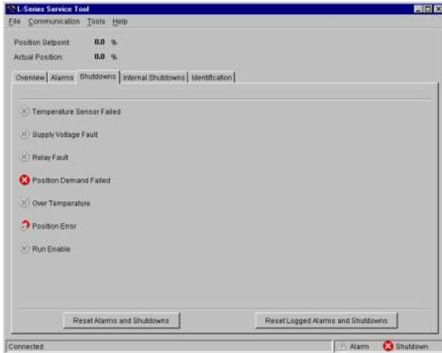
Figure 4-13. Service Tool – Shutdowns Tab
