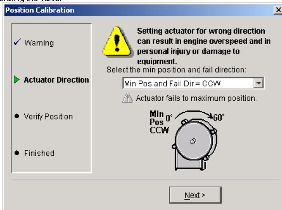
Figure 4-19. Service Tool—Manual Position Calibration
