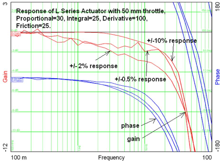
Figure 5-1. Bode Plot of L-Series Response
