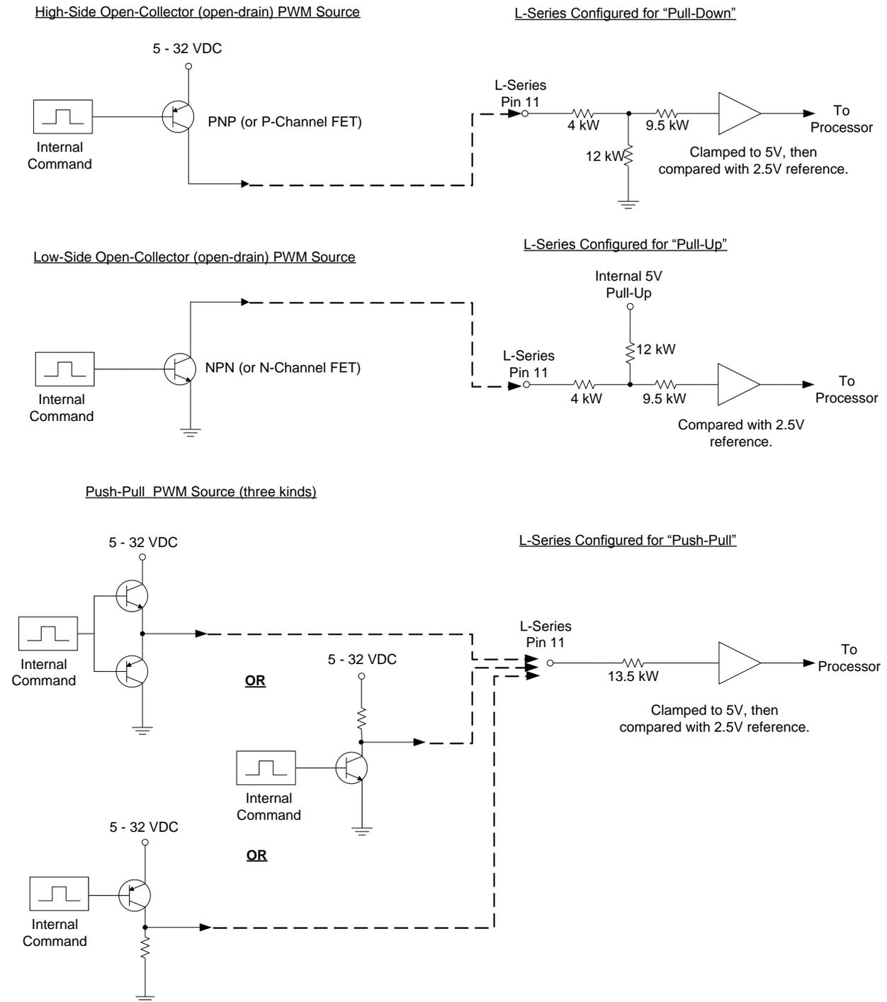
Figure 3-5. Acceptable PWM Input Types
