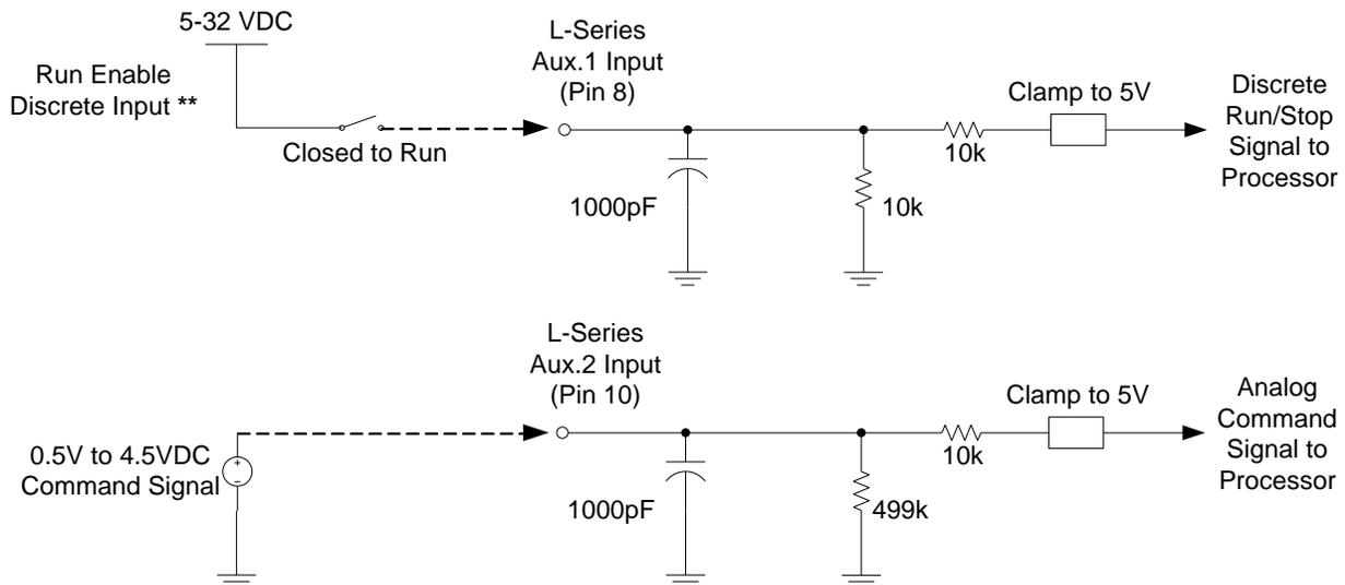
\*\* if optional external Run Enable is chosen during L-Series configuration, Aux. 1 can be used to enable or disable the actuator output shaft torque.
