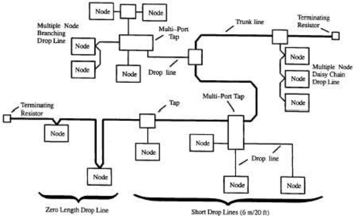
Figure 3-8 CAN System Wiring Example
