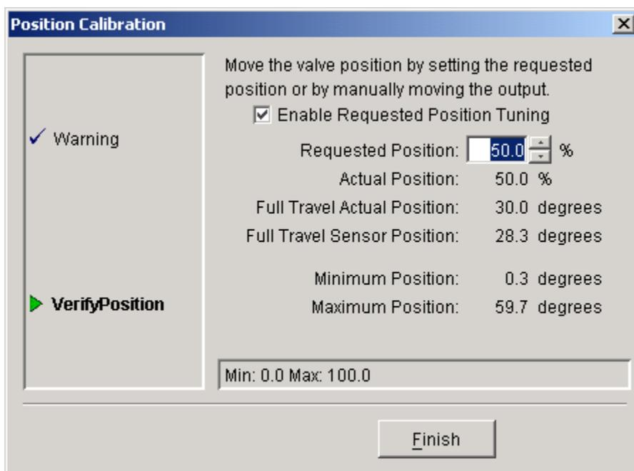
Figure 4-18. Service Tool—Verify Position Calibration
