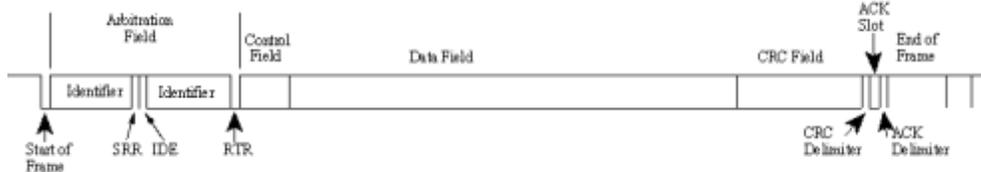
Figure 2-8. CAN 2.0B ("extended CAN") Data Frame
