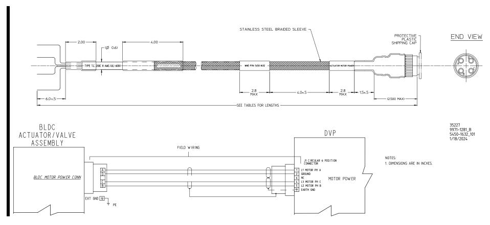
Figure 3-10. Cable, 4-Pin Motor Power
