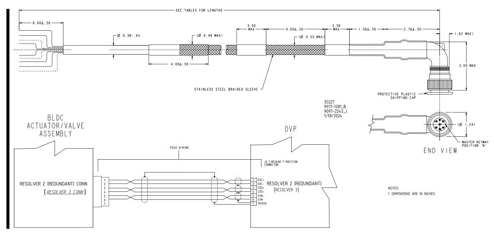
Figure 3-13. Cable, 7-Pin Actuator Motor Resolver #2 (Redundant)
