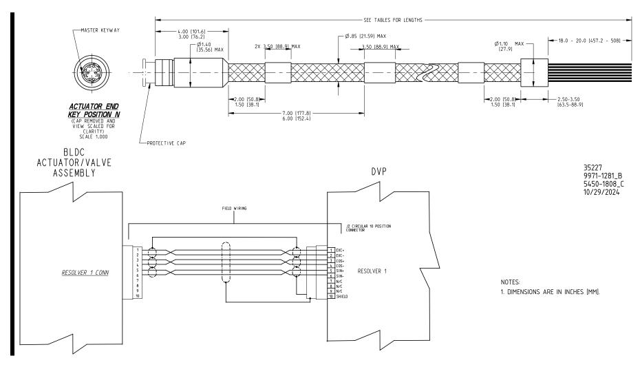
Figure 3-14. Cable, 10-Pin Actuator Motor Resolver #1
