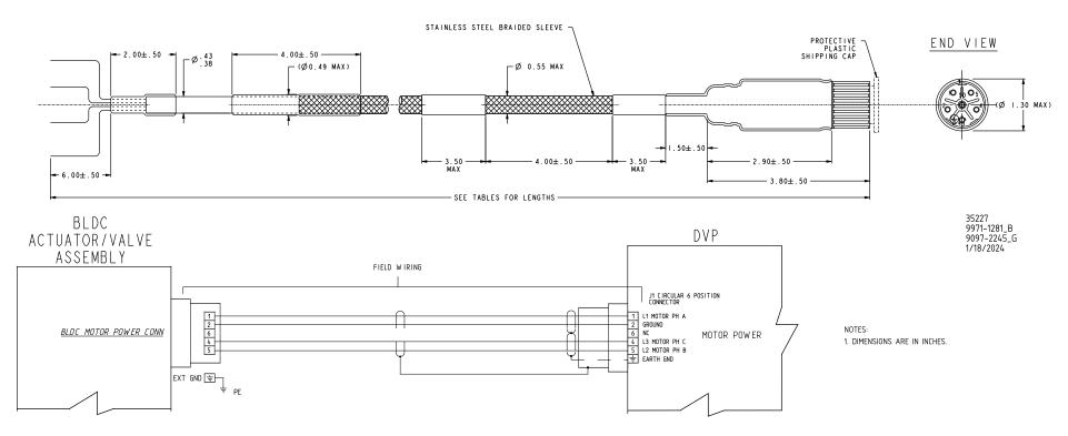
Figure 3-9. Cable, 6-Pin Motor Power Straight Connector at Actuator to Flying Leads at DVP J1 Connector, for ELA7, ELA13 with DVP5000
