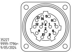
PIN 1 VA+ PIN 1 PIN 2 PIN 3 PIN 4 PIN 5 PIN 6 PIN 7 VA-VB+ VB-EXC+ EXC -POW ER PIN 8 PIN 9 GROUND GROUND ID CAN 3 H ID CAN 3 L SEAL PLUG SEAL PLUG SEAL PLUG SEAL PLUG PIN 9 PIN 10 PIN 11 PIN 12 PIN 13 PIN 14
