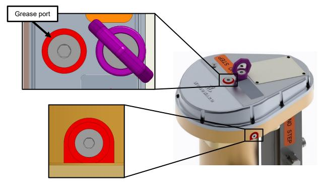
Figure 3-1. Grease Port Locations for ELA7 & ELA13 Actuators
