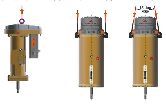
Figure 3-3. Vertical Lifting (ELA7 & ELA13 left, ELA53 right)
