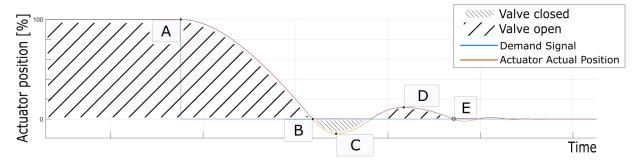
Figure 2-2. Failure Mode
