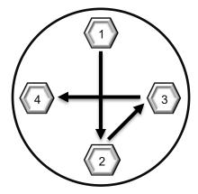
Figure 3-5. Interface Plate Fasteners 4-point Tightening Sequence
