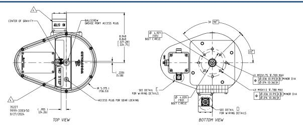
Figure 1-2c. ELA7 & ELA13 Outline Drawing (Top and Bottom View)
