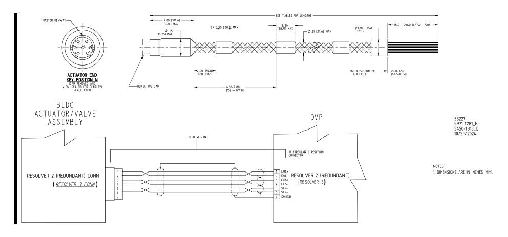
Figure 3-15. Cable, 7-Pin Actuator Motor Resolver #2 (Redundant)
