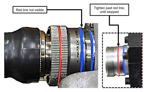
Figure 3-8. ID Module/Shaft Resolver Actuator Connector **Note:** Actual connector location on actuator may appear different than that shown.
