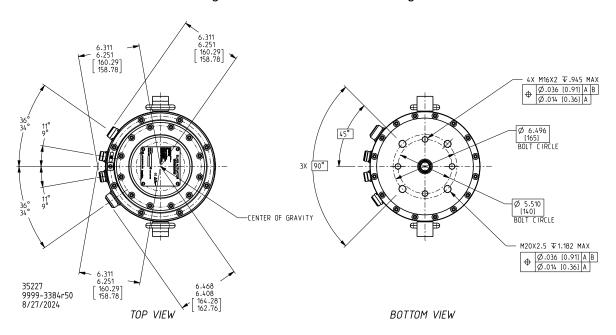
Figure 1-3c. ELA53 Outline Drawing (Top and Bottom View)
