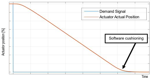
Figure 2-1. Actuator Response to a Step Demand
