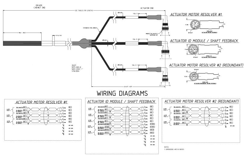
Figure 3-16. Integrated Signal Cable
