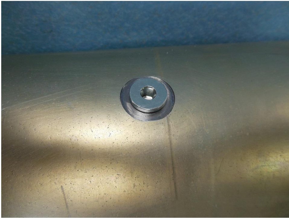
Figure 1-5. Actuator Body Grease Port with Plug Installed
