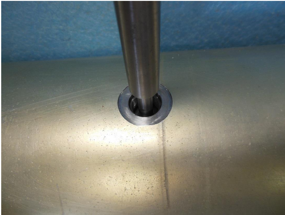
Figure 1-8. Body Grease Port with Greasing Adaptor Installed
