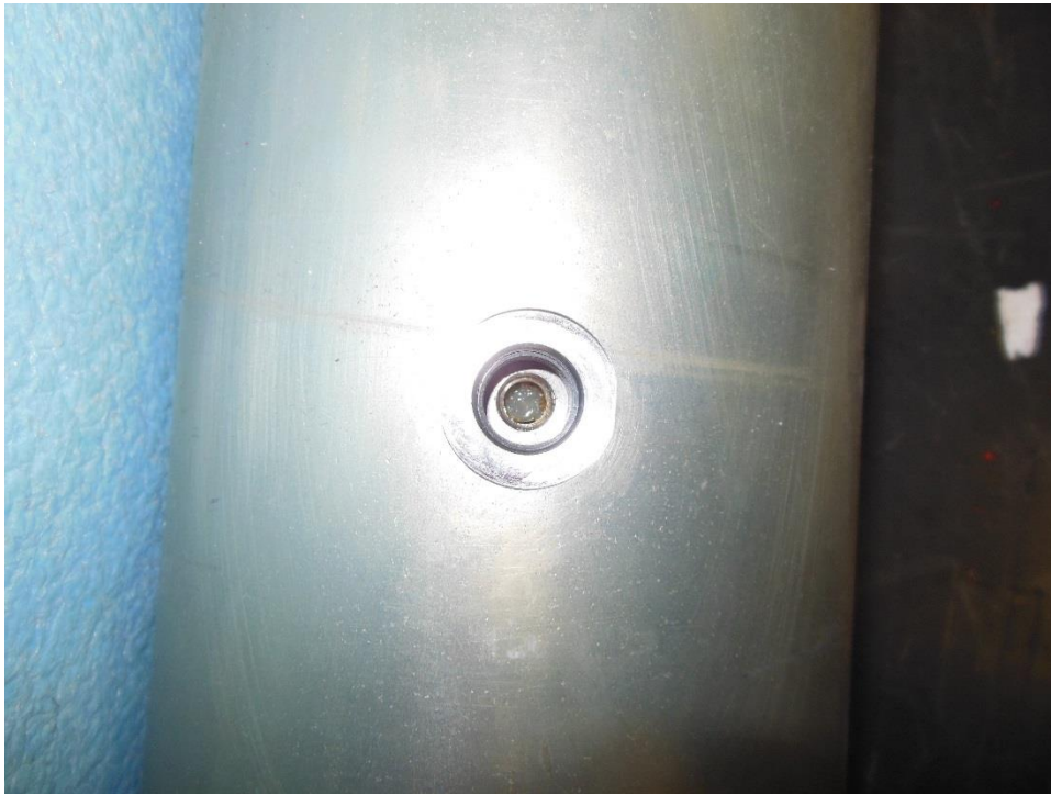
Figure 1-7. Body Grease Port Unplugged
