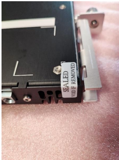
Appendix A-5. Intact Seal on Chassis
