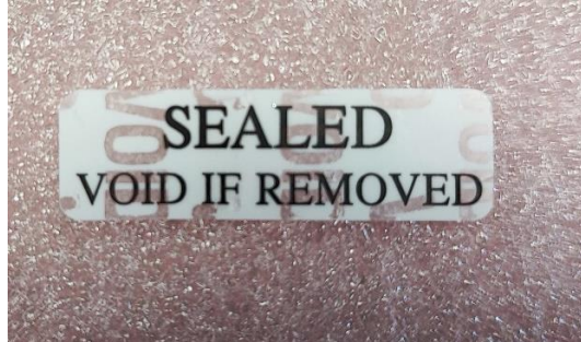
Appendix A-4. Seal That Has Been Tampered With
