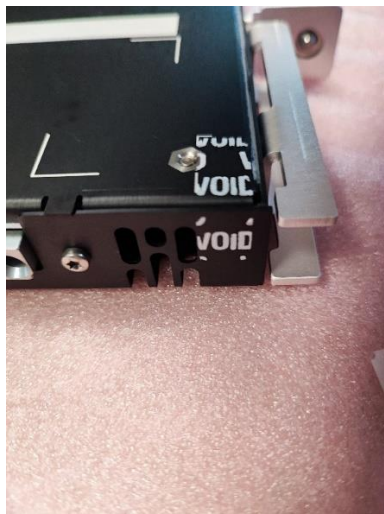
Appendix A-6. Tampered Seal on Chassis
