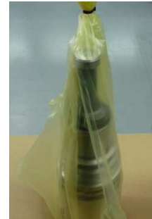
Close VCI foil with cable tie
